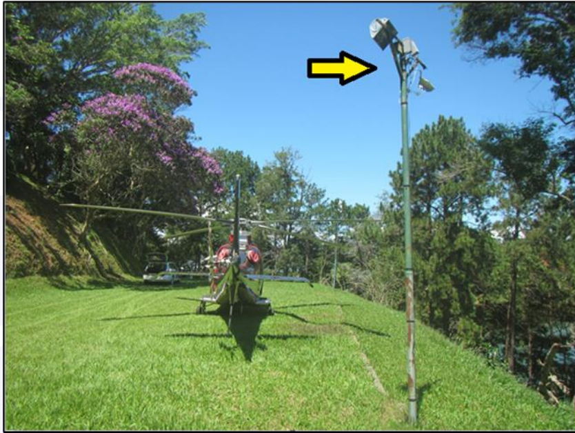
Figure 1 - Final position after the occurrence and highlighting the lighting pole hit by the tail rotor.
