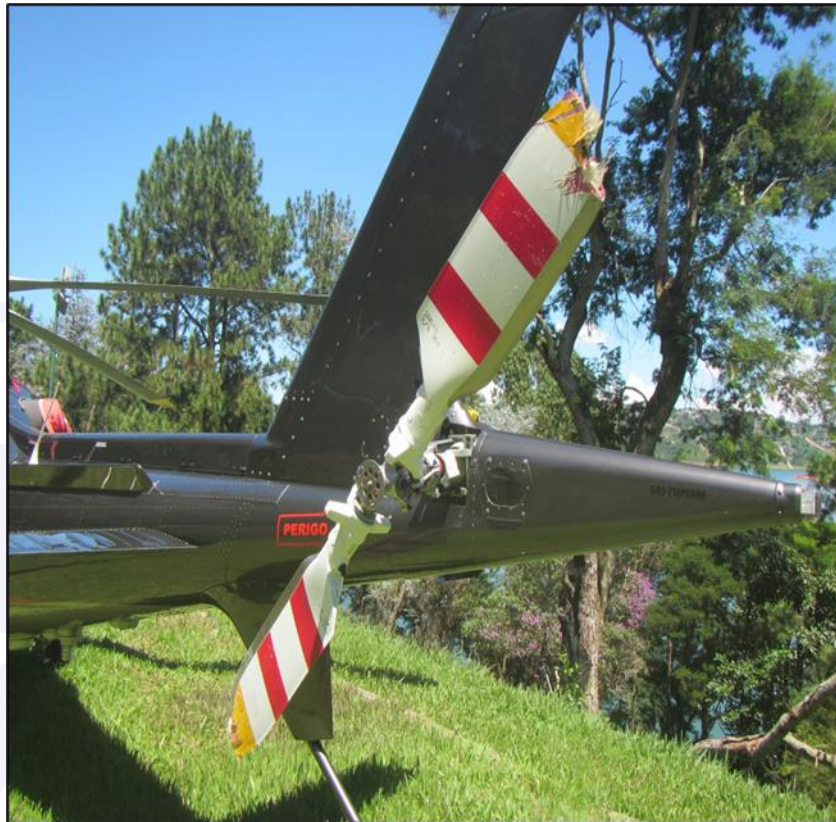
Figure 3 - Detail of damage to the tail rotor.
