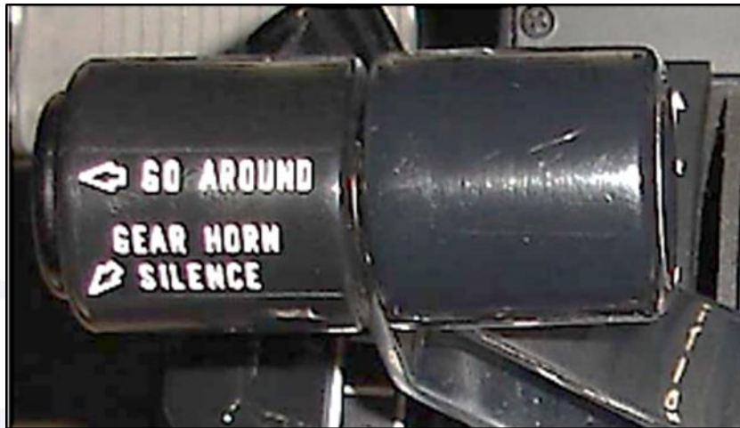
Figure 13 - Horn silence button of the landing gear configuration.
