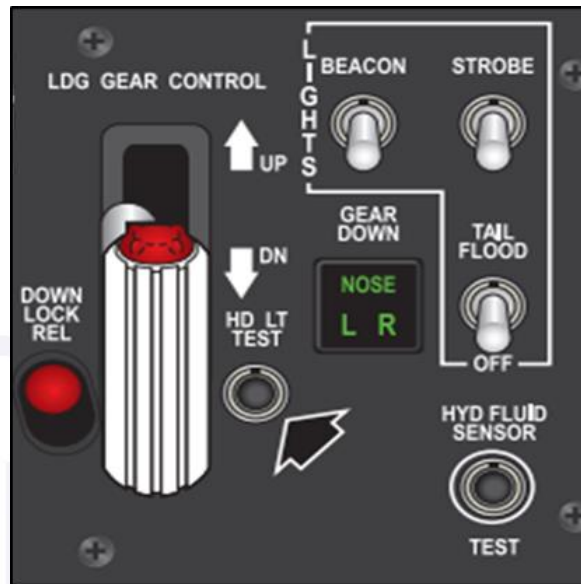
Figure 12 - HD LT TEST button used to check the red control lights on the landing gear lever.
