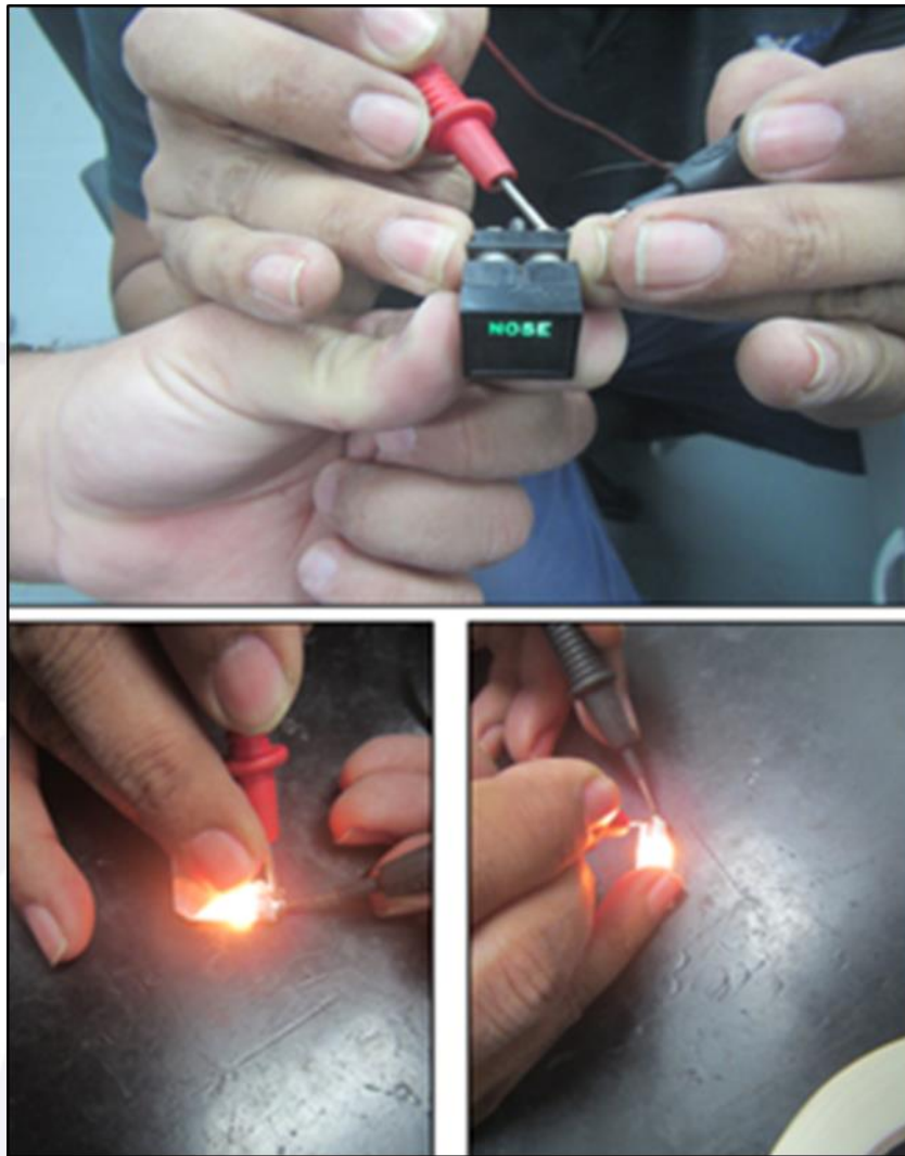
Figure 39 – Testing the lights of the nose landing gear position indicator.
