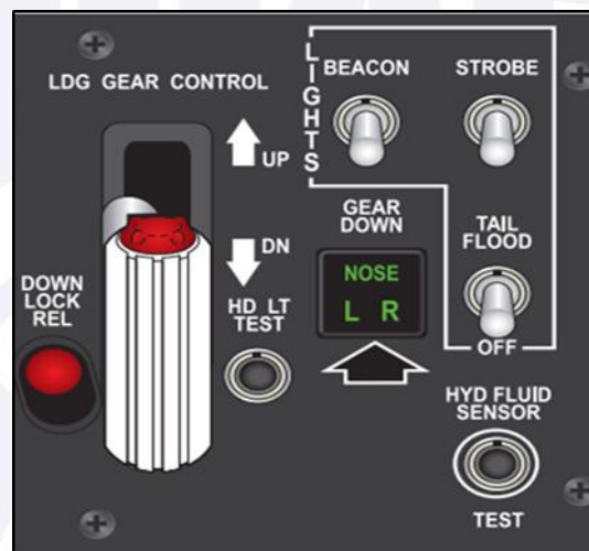
Figure 10 - Landing gear position selector and landing gear position indicator lights.
