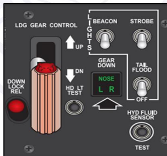
Figure 11 - Landing gear control lever handle (red light indicates landing gear in transit).
