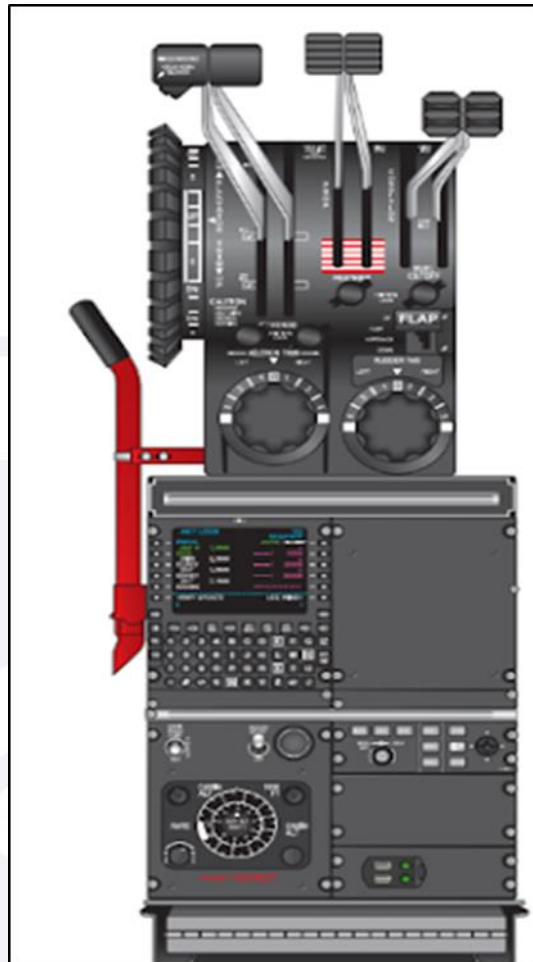
Figure 8 - Emergency actuation lever highlighted in red (LANDING GEAR ALTERNATE EXTENSION).
