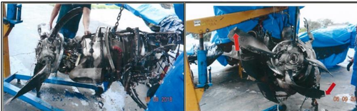
Figure 33 - View of the engine and right propeller, showing the blades with forward bending.
