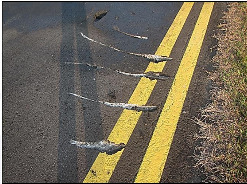
Figure 22 - Cuts in the asphalt made by the propeller blades of the right engine.
