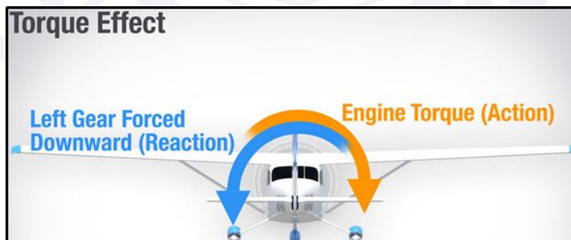
Figure 57 - Torque effect acting on a single-engine propeller-driven aircraft. Source: image from the website www.boldmethod.com .
