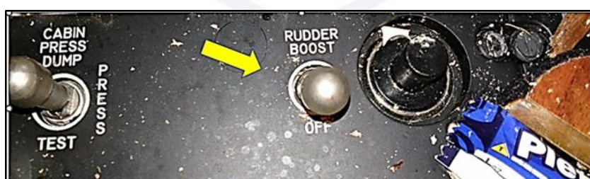
Figure 27 - Position of the Rudder Boost System switch, as found amid the wreckage.
