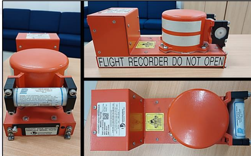
Figure 19 - Image of the CVR of the PP-SZN airplane.
