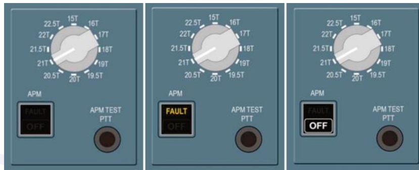
Figure 10 - ATR-72-212A APM Control Panel set to 21T under three conditions: Normal (ON), Fault (FAULT), and OFF indications (respectively).
