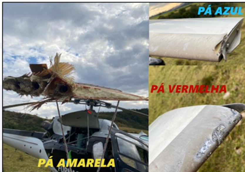
Figure 2 - Damage to the main rotor blades.
