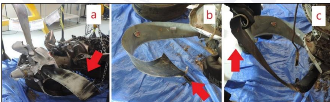
Figure 10 - (a) propeller, general appearance and perpendicular marks; (b) blade tip severed by impact with a tree; and (c) bent blade tip.
