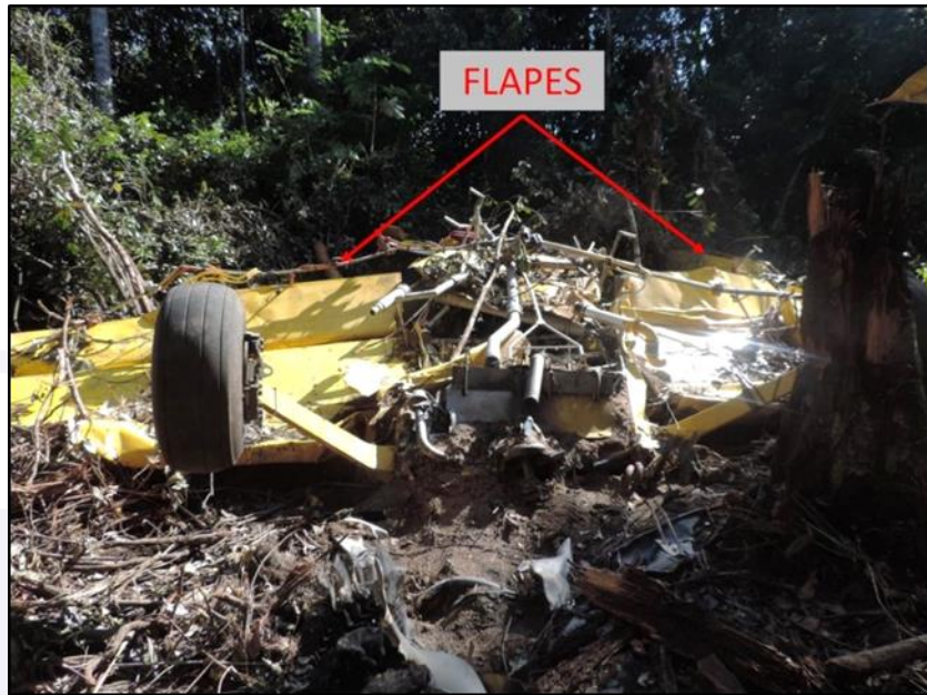
Figure 2 - Front section of the aircraft buried in the ground, and position of the flaps.
