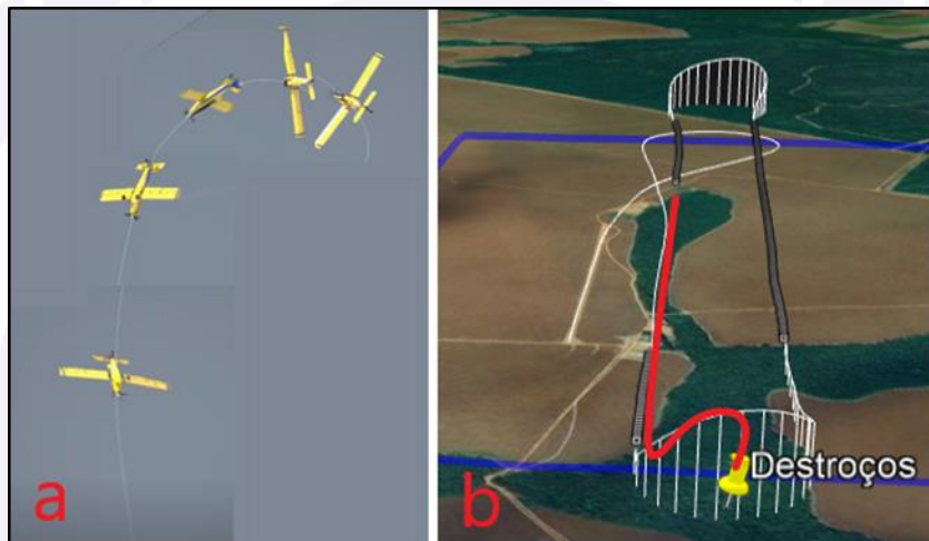
Figure 14 - spin image (a); and image of the estimated final flight trajectory (b) in red.
