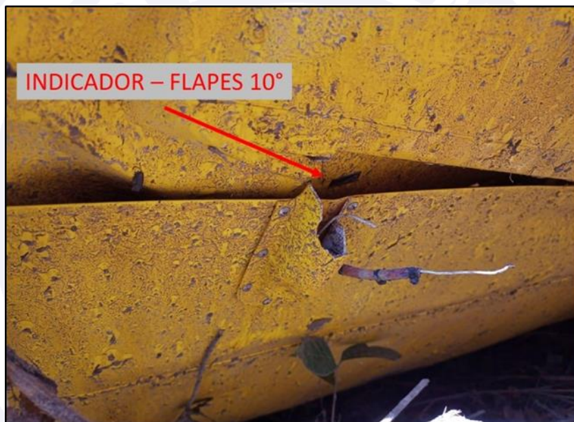
Figure 3 – Rectangular mark indicating flaps at 10^\circ .
