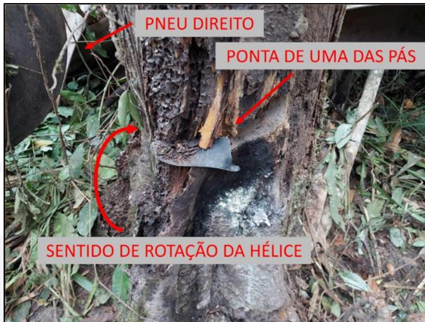
Figure 4 - Tip of the blade of one of the propellers embedded in a tree trunk.
