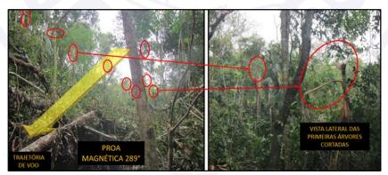
Figure 12 - Aircraft trajectory at the accident site.
