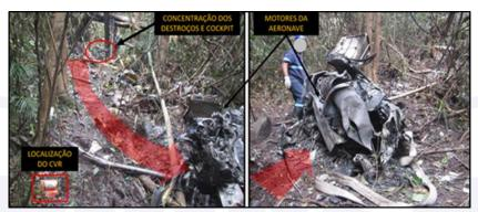
Figure 13 - View of the engines and location of the CVR, in relation to the cockpit.
