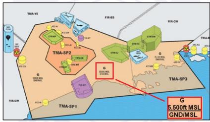
Figure 24 - Plan view of the TMA-SP, highlighting the "G" class airspace.
