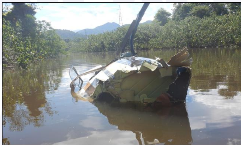
Figure 3 - Overview of the damage sustained by the helicopter (detail of the transmission line towers in the background).
