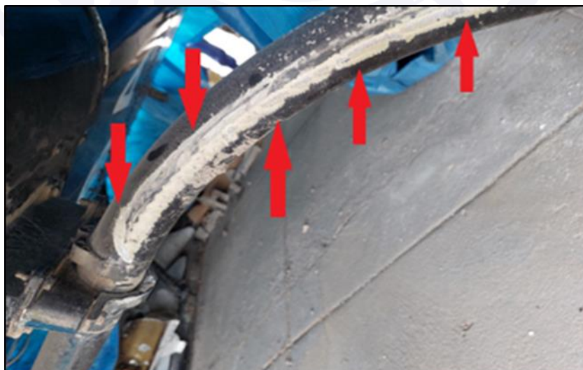
Figure 4 - Marks of the impact against the transmission line cables.
