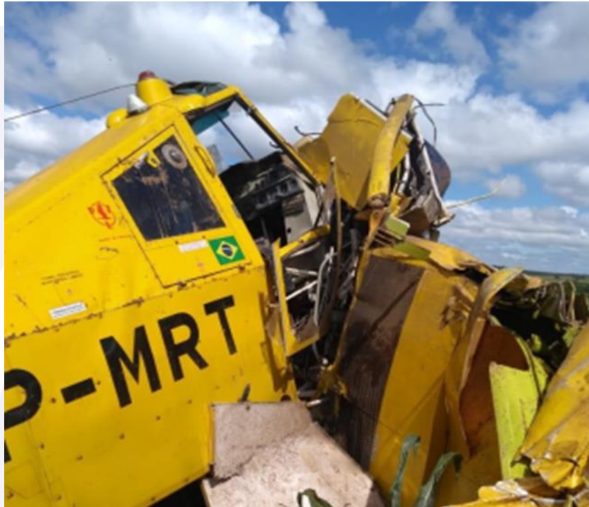
Figure 2 - Detail of the fuselage and cabin damage.
