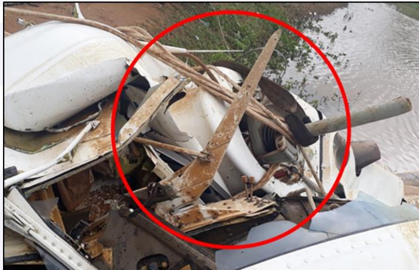
Figure 21 - Detail of the aircraft's lower wire-cutter with no traces of contact with the lightning-rod cable.
