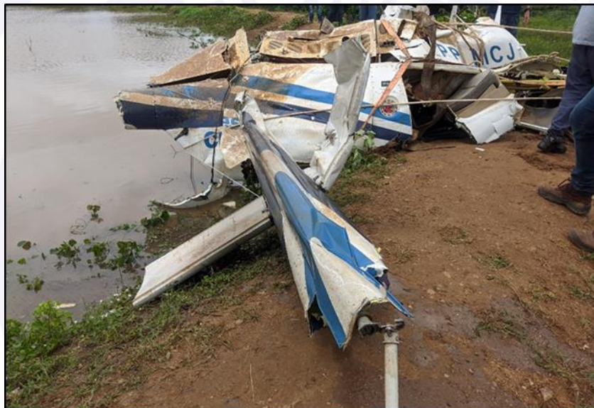
Figure 27 - Damage to the left-hand horizontal stabilizer, with sectioning of the tail boom and tail-rotor transmission shaft.
