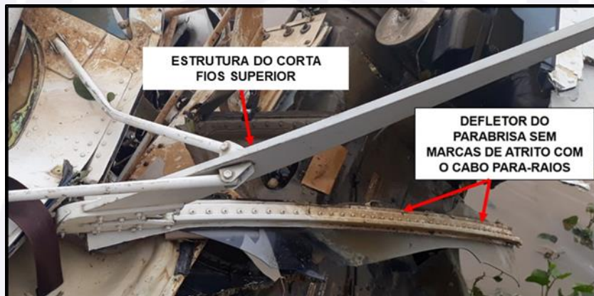
Figure 24 - General view of the upper wire-cutter with the central deflector of the windshield.
