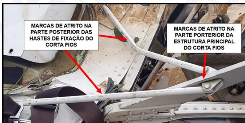
Figure 25 - General condition of the upper wire-cutter.
