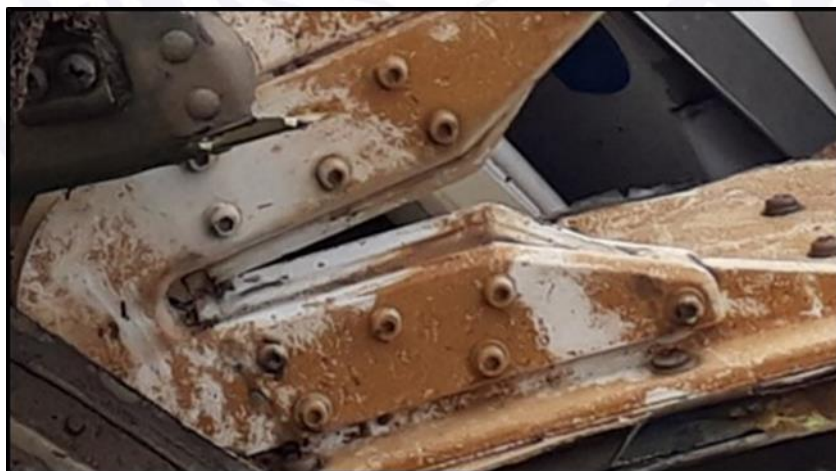
Figure 22 - Enlarged image of the aircraft's lower wire-cutter.
