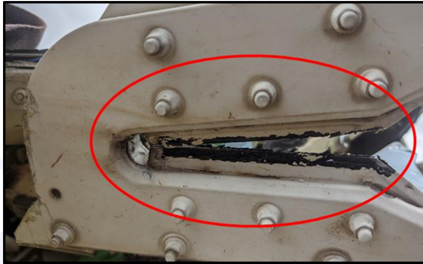
Figure 23 - Upper wire-cutter with evidence of contact with the lightning-rod cable.
