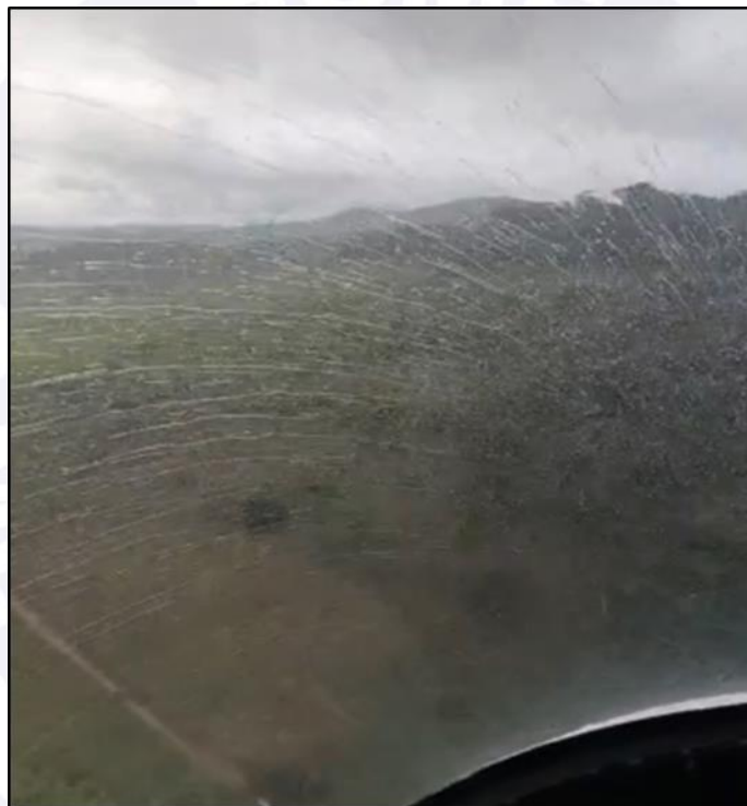
Figure 30 - Influence of rain droplets on the windshield of a helicopter, compromising the pilot's visibility. Source: Piloto Policial website.
