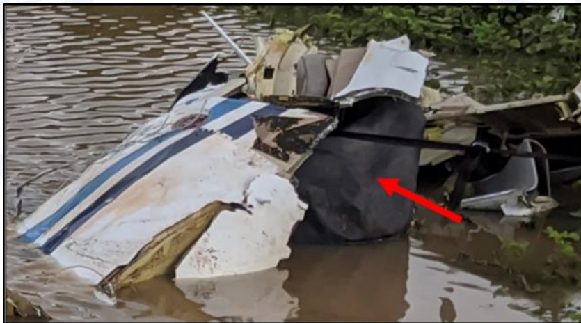
Figure 29 – Aircraft debris, with the fuel tank in highlight.
