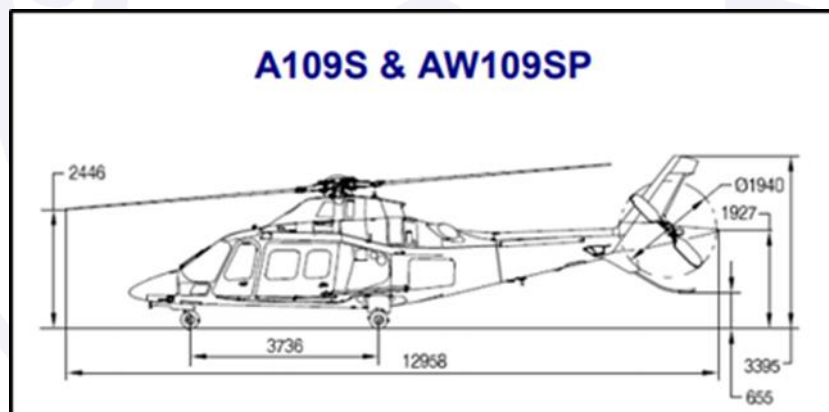
Figure 1 - Dimensions of the AW109SP, in millimeters.
