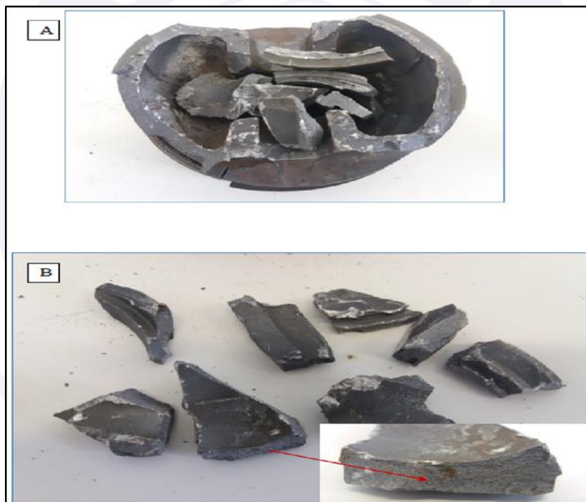
Figure 5 - General view of the piston and fragments. The red arrow indicates fractures attributed to an overload mechanism.
