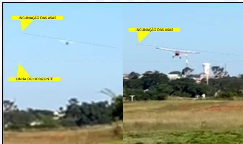
Figure 3 - In detail, the aircraft corrections to maintain alignment with the runway axis.
