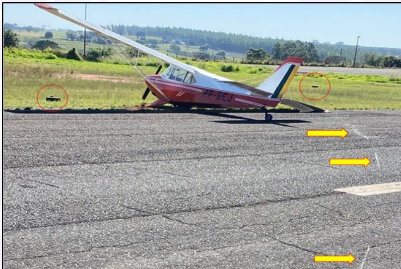
Figure 1 - Highlighted in the two red circles is the final position of the main gear wheels. The yellow arrows show the marks left on the asphalt by the right-hand wing tip.
