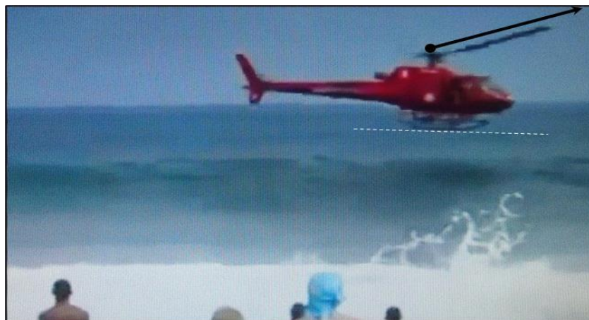
Figure 12 - Moment of landing of the aircraft at sea, highlighting the increase in the "cone effect" in the main rotor.
