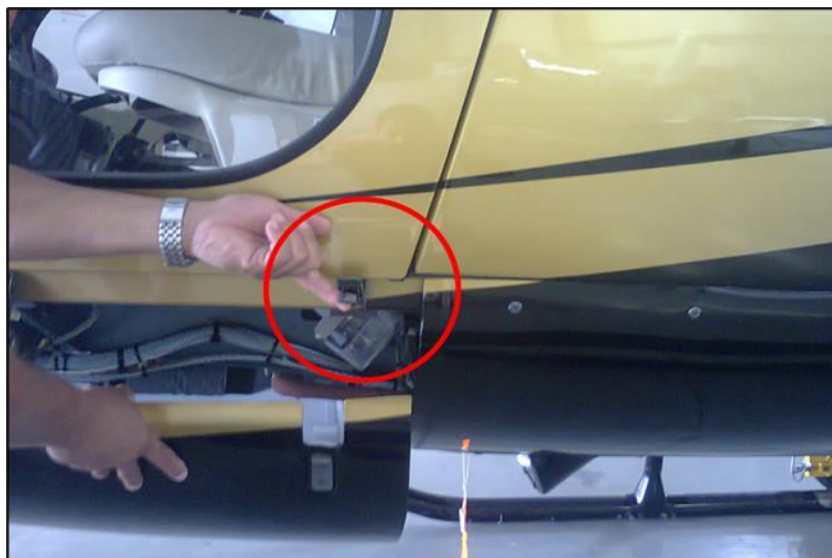
Figure 16 - Alignment of the lower fairing latch crack with the acrylic housing of the TWIST GRIP microswitches (photo of a helicopter of the same model).
