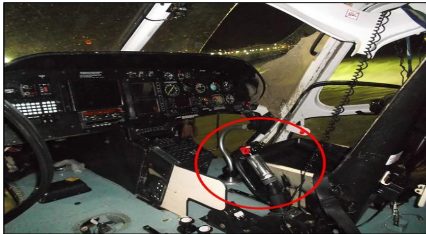
Figure 13 - Image of the cabin, shortly after removing the aircraft from the sea, highlighting the collective control in the fully pulled position.
