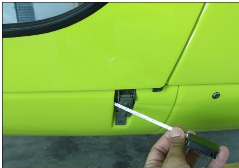
Figure 15 - Bottom fairing latch crack (photo of a helicopter of the same model).
