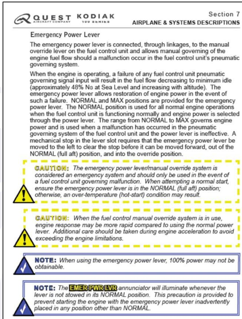
Figure 2 - Description of the Emergency Power Lever, extract from the Airplane Information Manual (Revision 18, October 2016).
