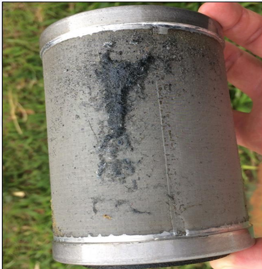
Figure 4 - Debris found in the fuel airframe filter.
