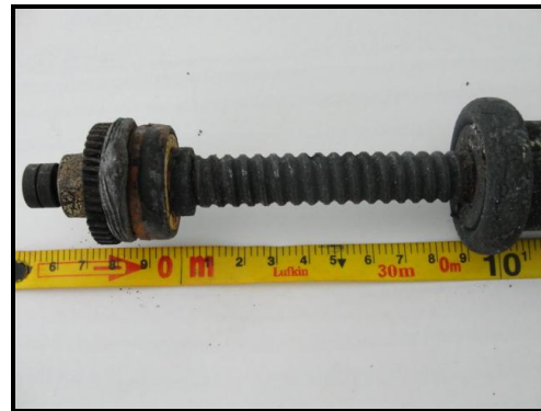
Figures 5 and 6 - Comparison between the endless screw of the flap in an aircraft with fully extended flaps and the endless screw of the accident aircraft.
