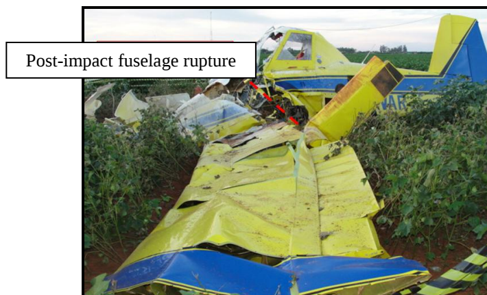
Figure 4 – Post-impact fuselage breakage.
