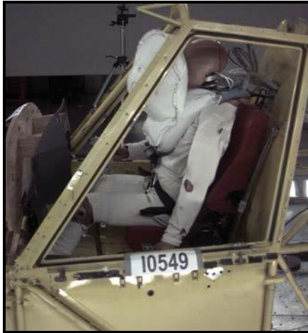
Figure 6 – Use of a crash test dummy to show the functionality of the AT-502B aircraft airbag.
