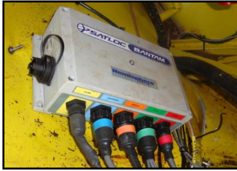
Figure 1 - CPU of the PR-VAR aircraft GPS.
