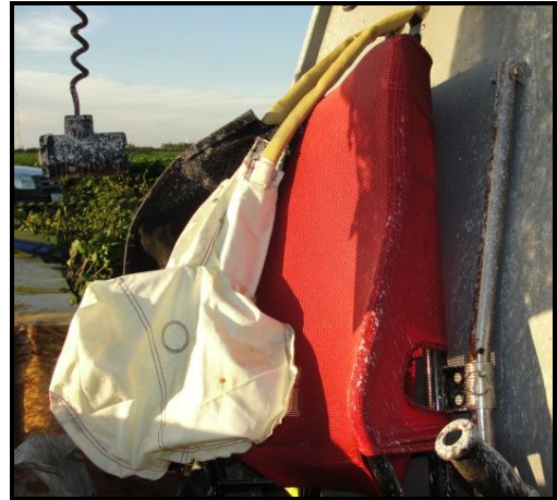
Figure 7 – Picture showing that the airbag of the PR-VAR was activated.
