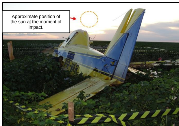
Figure 9 – Breakage of the left horizontal stabilizer as a result of the impact.
