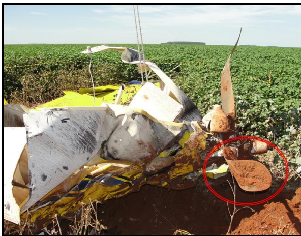
Figure 8 – Propeller blade highlighted by the red circle, indicating that the engine was developing high power at the moment of impact with the ground.
