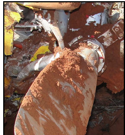
Figure 8 – Propeller blade highlighted by the red circle, indicating that the engine was developing high power at the moment of impact with the ground.
