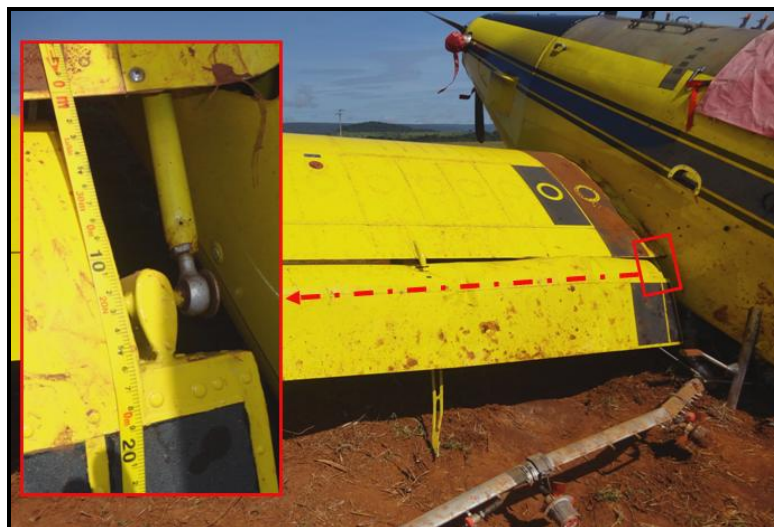
Figure 5 – Measurement made on the left-hand side flap panel, showing a distance of 17.7cm up to the rivets of the lower part.
