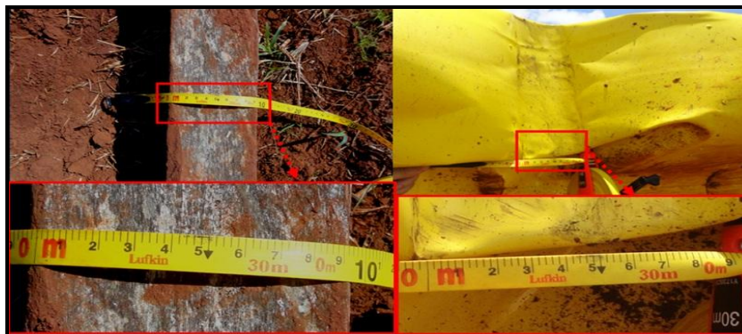
Figure 3 – On the left, the fence post with a width of 9 cm. On the right, the mark left by the post on the left-wing leading edge (second impact).
