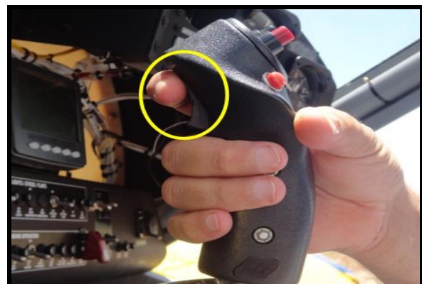
Figure 13 – Command for retracting the flaps.
