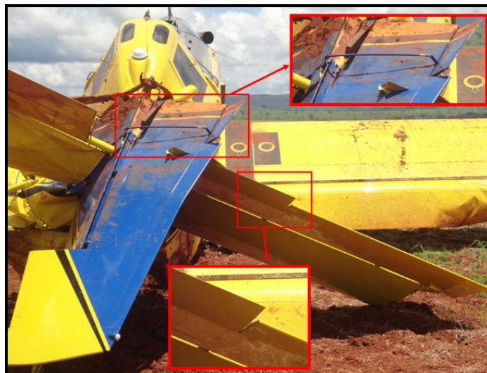
Figure 7 – Position of the rudder and elevator trimmers.
