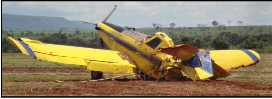
Figure 9 – Damage to the rear section of the aircraft.
