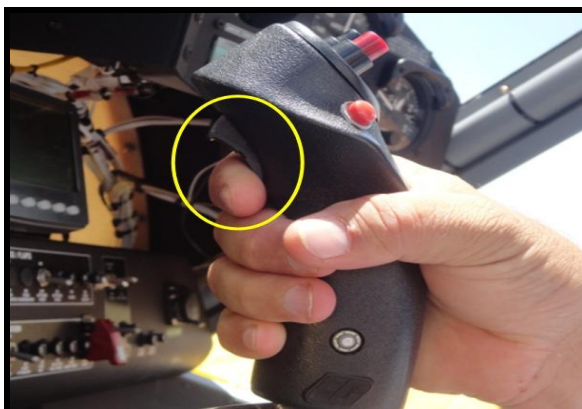
Figure 12 – Command for flaps extension.
