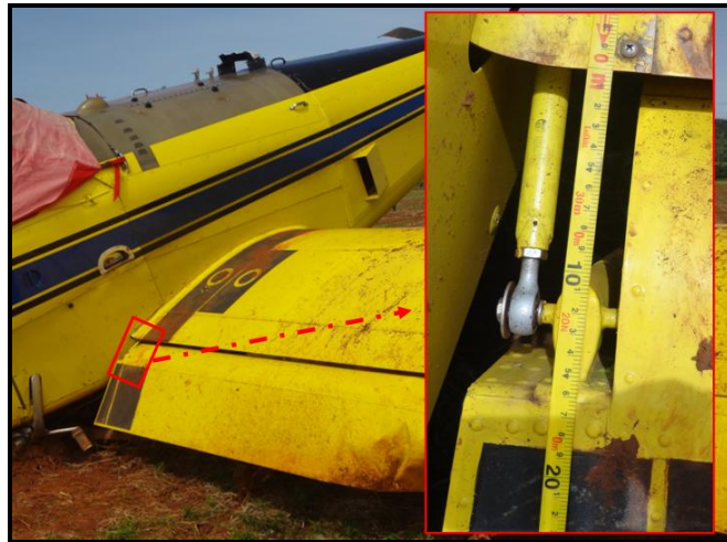
Figure 6 - Measurement made on the right-hand side flap panel, showing a distance of 17.7cm up to the rivets of the lower part.
