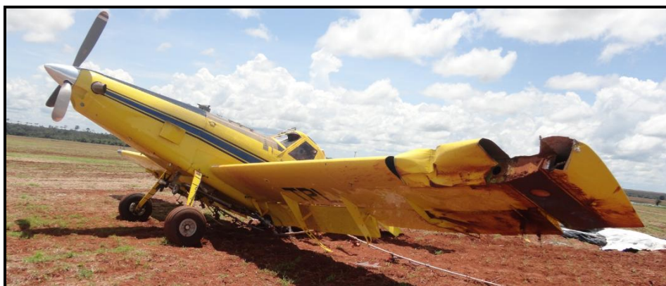
Figure 8 – Damage to the left-wing leading edge.
