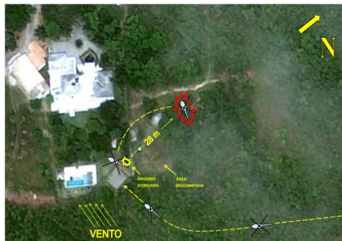
Figure 10 – Trajectory of the helicopter from the approach for landing up to the collision with the ground.
