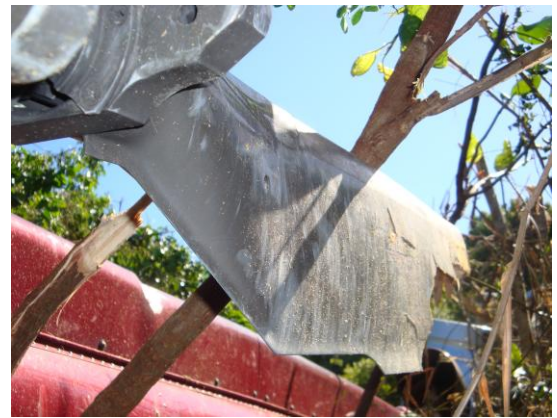
Figure 12 – Damage to the tail rotor blades.
