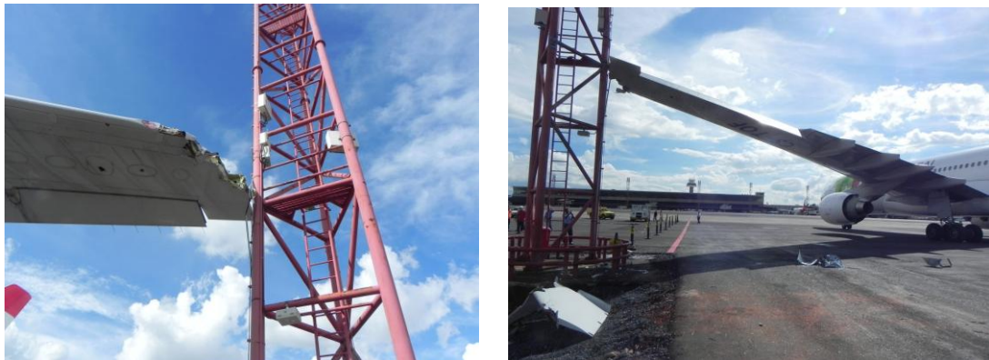
Figures 2 and 3 – Aircraft situation after the collision.
