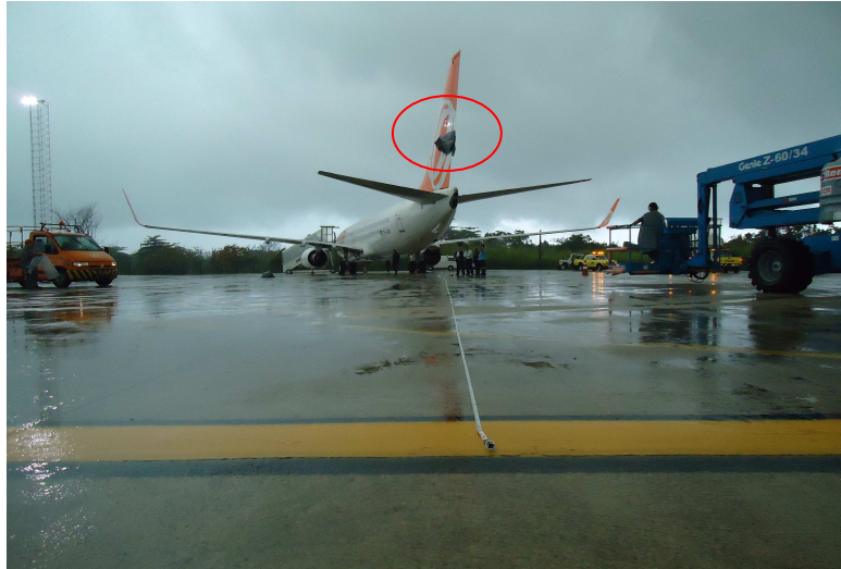
Figure 6 – Damage to the vertical stabilizer of the B737 after the collision. In the foreground, the yellow line along which the B777 was taxiing in.
