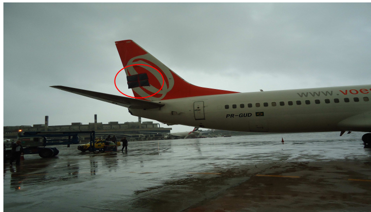
Figure 7 – Aspect of the damage to the vertical stabilizer of the B737 after the collision.
