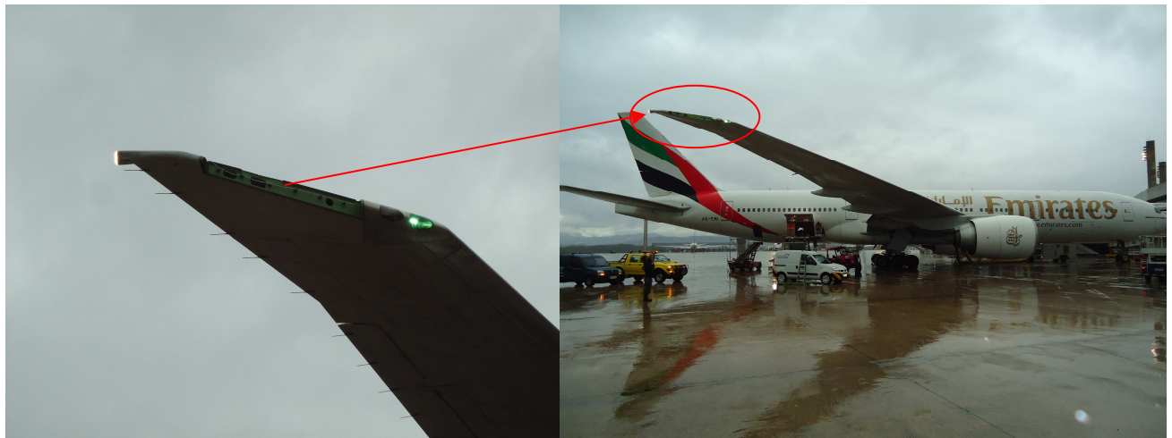
Figures 4 and 5 – Damage to the right wing tip of the B777 aircraft after the collision.
