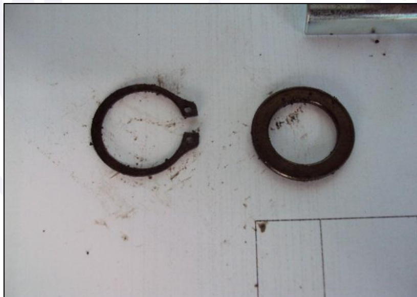
Figure 4 – Ring and washer found loose in the oil sump.
