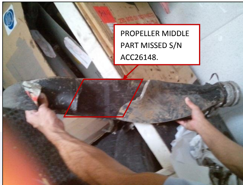
Figure 11 – Fractured propeller blade.
