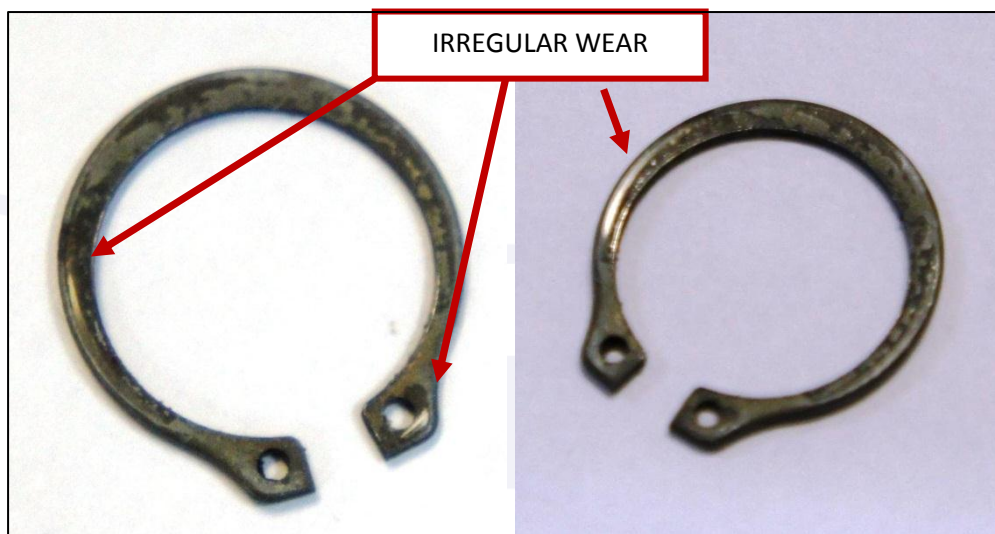
Figure 7 - External retaining ring (P/N STD-1737) with marks of rubbing.
