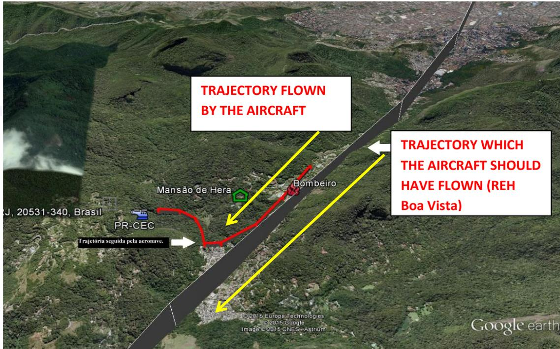
Figure 2 – Trajectory flown by the aircraft until radar contact was lost.
