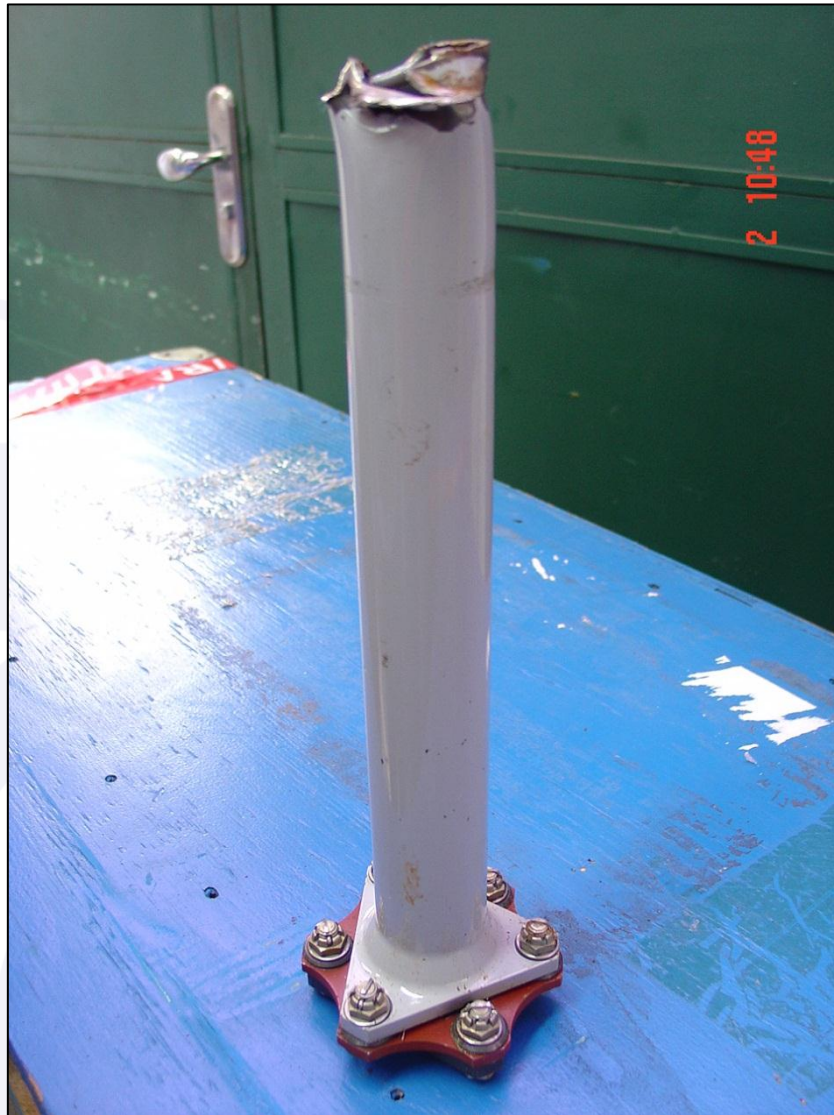
Figure 5 – Connecting shaft between the engine and the main box showed rupture close to the point of attachment to the main box.
