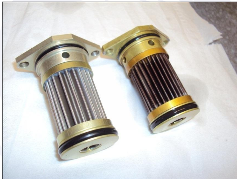
Figure 2 – on the right, a filter removed from the aircraft FCU, compared with a brand new one (on the left).
