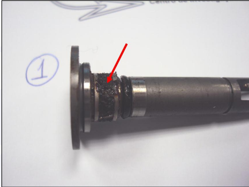
Figure 5 – View of the NG piston with lots of contamination in the fuel filter.
