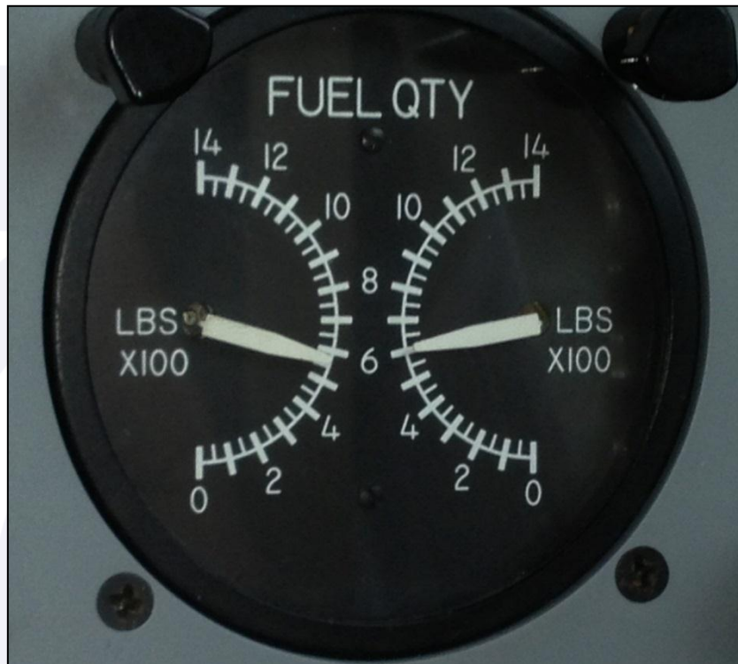
Figure 8 – Initial indication of the fuel gauge (1,200 lb.).
