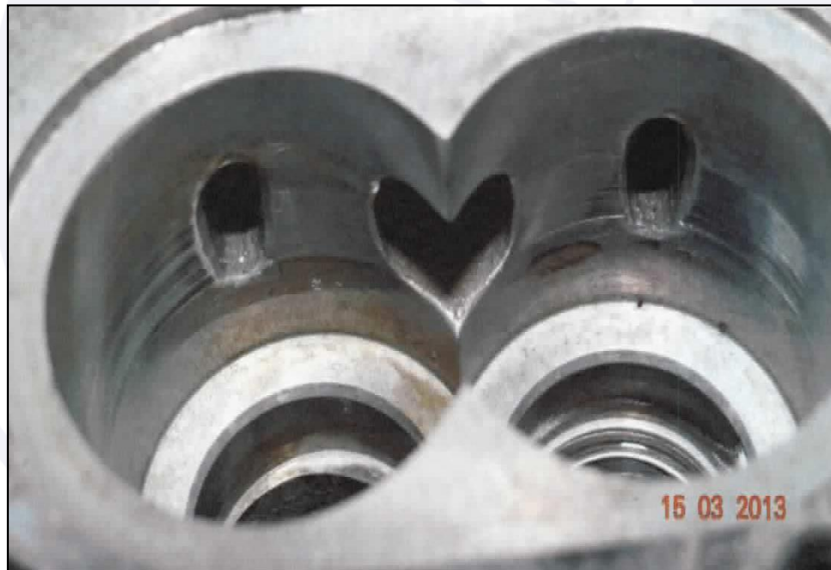
Figure 1 – View of the fuel pump frame, showing marks of rubbing in the housing of gears.
