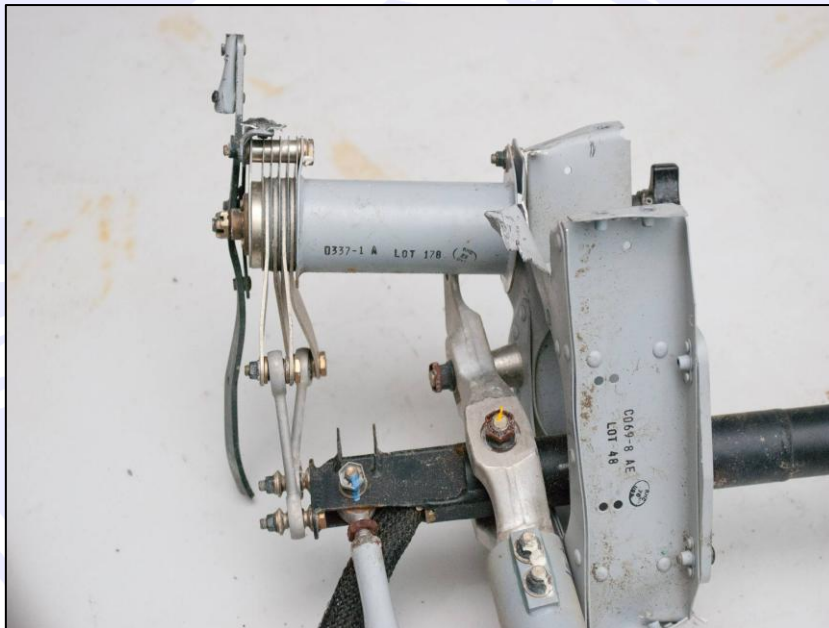
Figure 23 – Bending and deformation in the movable parts of the cyclic control caused by overload.
