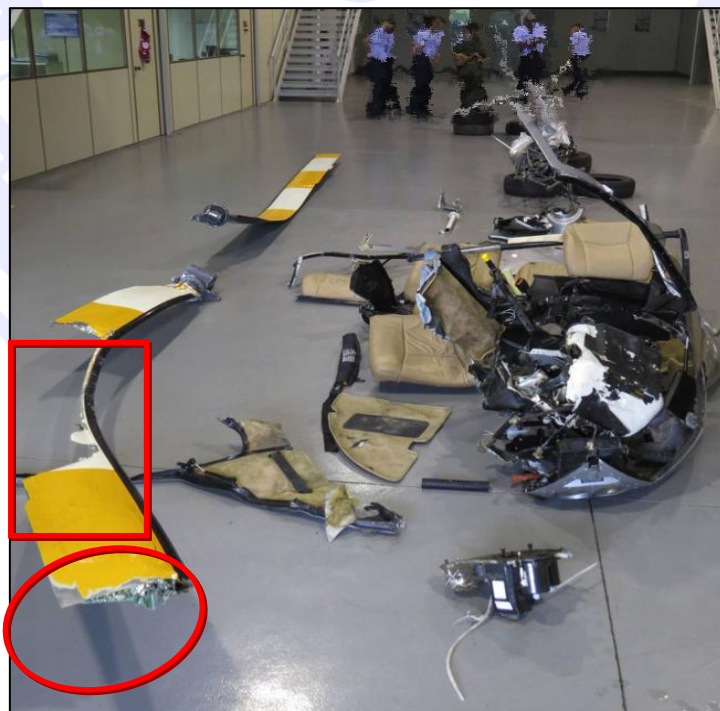
Figure 11 – Leading edge of the blade showing curvature in the direction of rotation, absence of material of the blade profile, and a fracture perpendicular to blade length.
