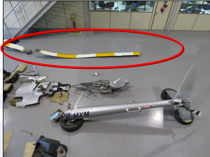
Figure 9 – Main rotor blade deflected upward.
