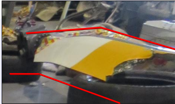
Figure 10 – Main rotor blade deflected downward.
