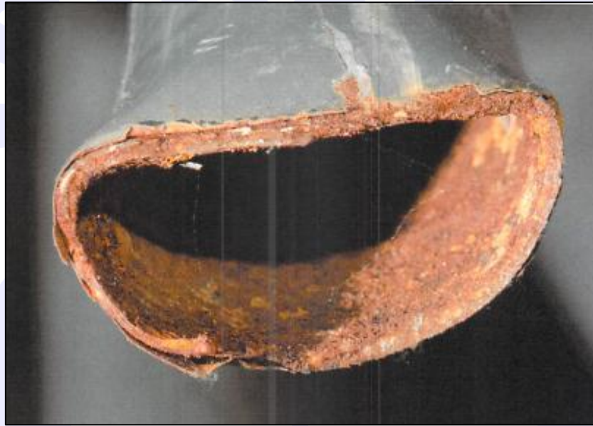
Figure 29 – Frame tube broken as a result of overload, with “fishmouth” type deformation at the point of breakage.
