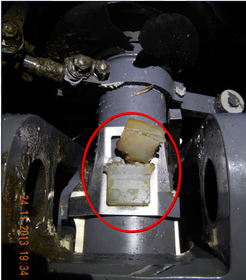
Figure 13 – Broken teeter stop of the main rotor head.
