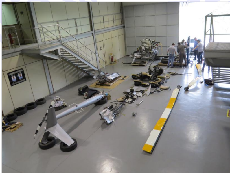
Figure 6 – 2D-reconstruction of the aircraft in the SERIPA III hangar.
