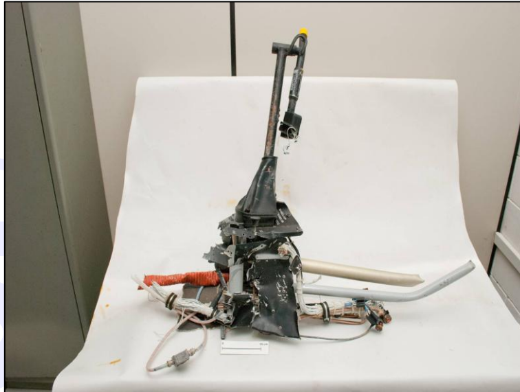
Figure 19 – Cyclic control assembly, including the friction adjustment mechanism, sent to the DCTA.
