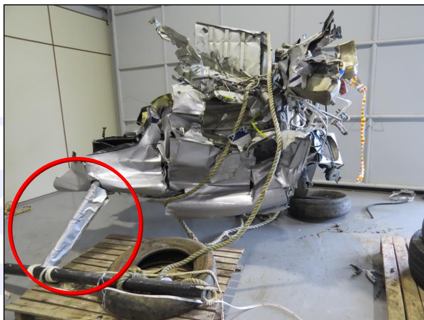
Figure 14 – Forward strut fairing with deformation.
