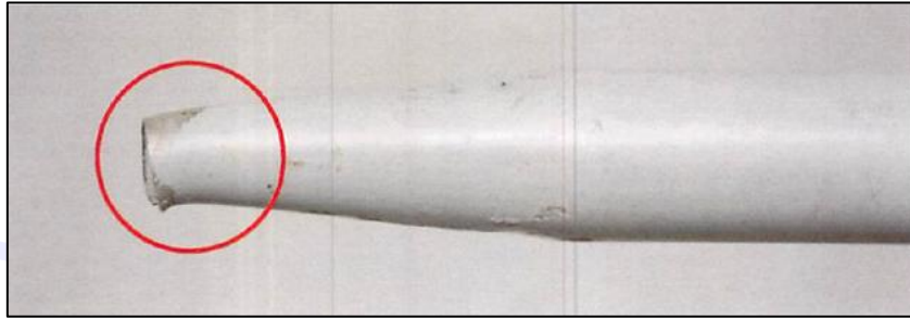
Figure 28 – Flight control tube broken as a result of overload, showing plastic deformation.
