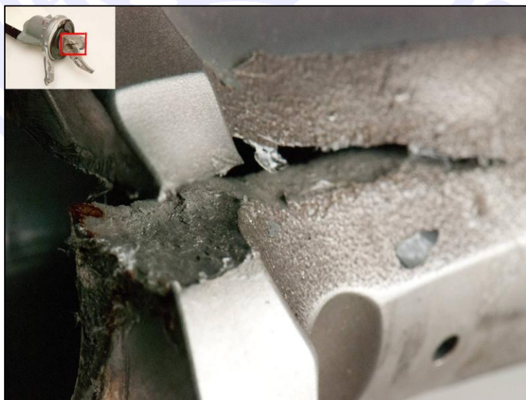
Figure 21 – Blade spindle fracture surface.
