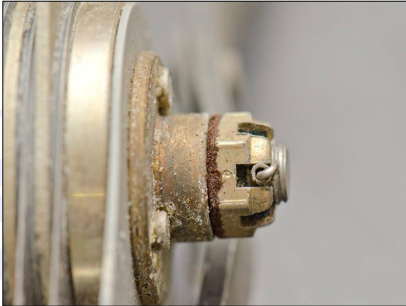
Figure 24 – Cyclic friction adjustment bolt at the counterclockwise stop: no friction applied.
