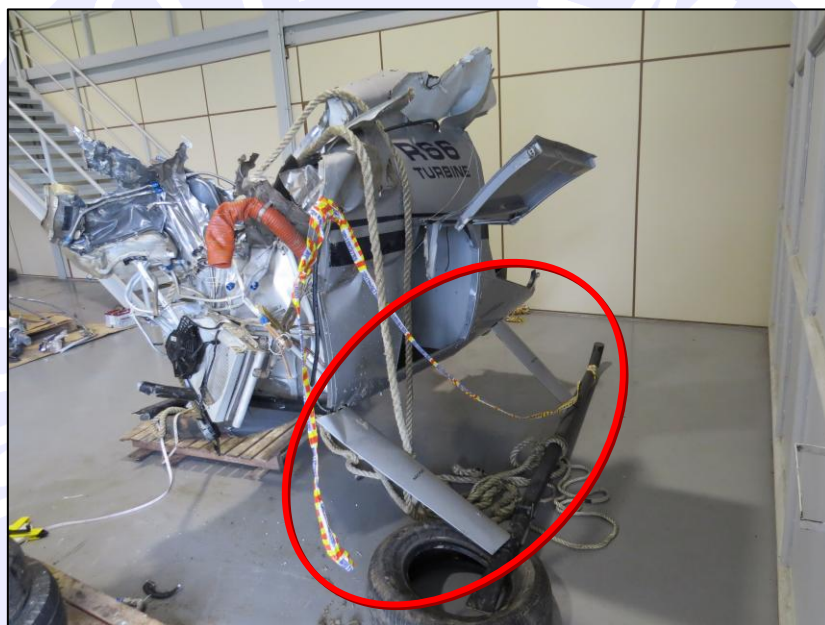
Figure 15 – Strut fairing of the right skid and part of the fuselage with little damage.
