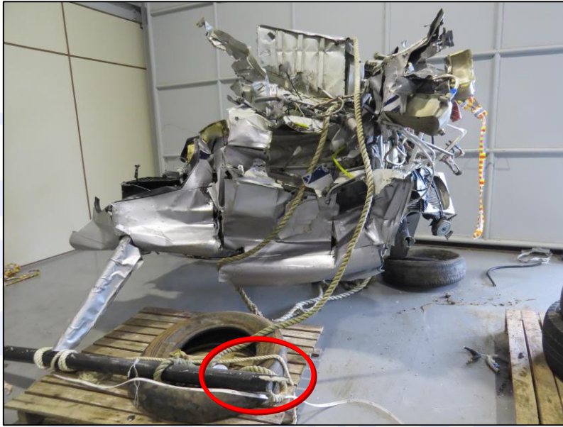
Figure 12 – Left ski with a breakage in the back part.
