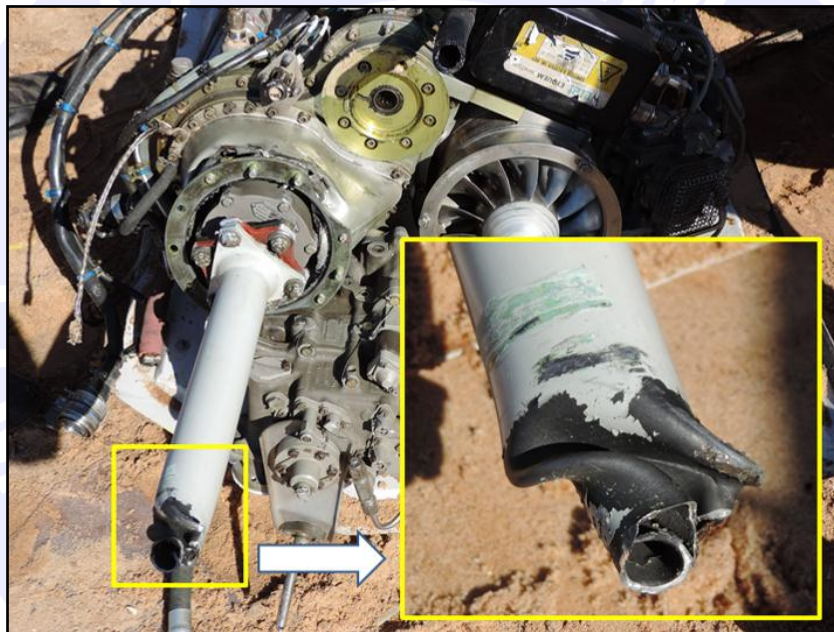
Figure 16 – Main rotor activation shaft connected to the engine. In highlight, the point of fracture.
