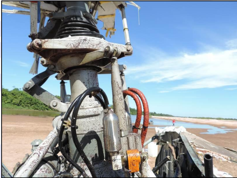
Figure 38 – Dirt adhered to the places where the hydraulic fluid spread on the main rotor mast during the impacts.
