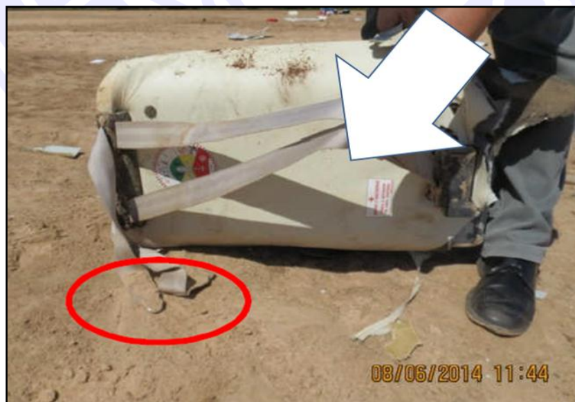
Figure 27 – Suspenders of the right front seat (pilot's) not fastened.
