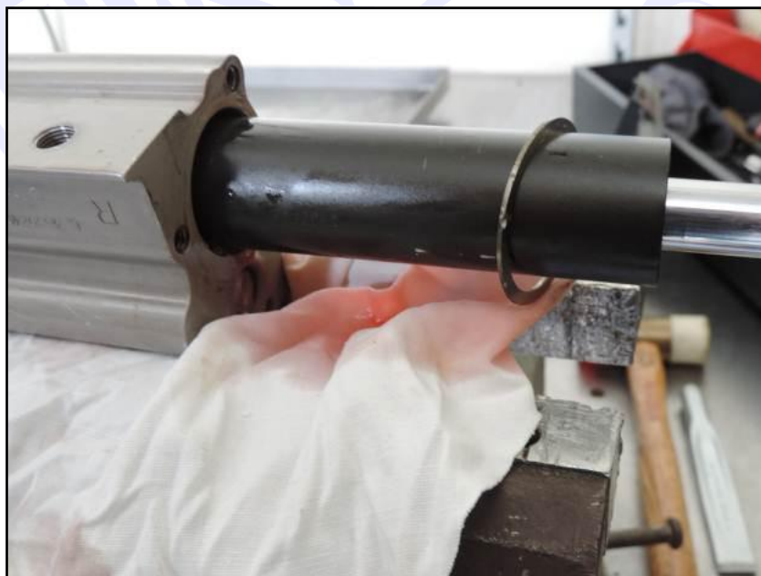
Figure 43 – Disassembly of the left servo control.
