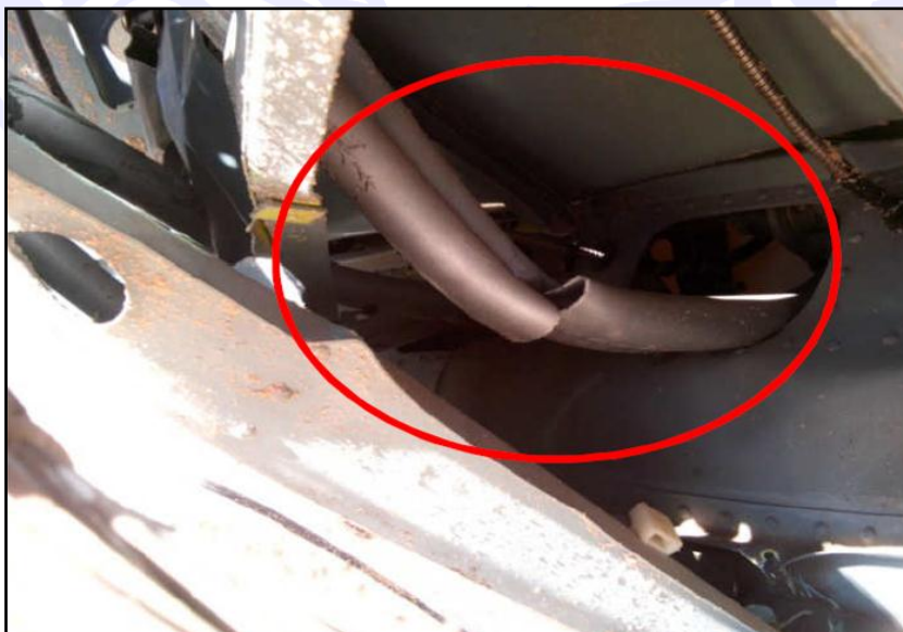
Figure 37 – Lateral cyclic and collective control levers on the left side of the lower part of the cabin.
