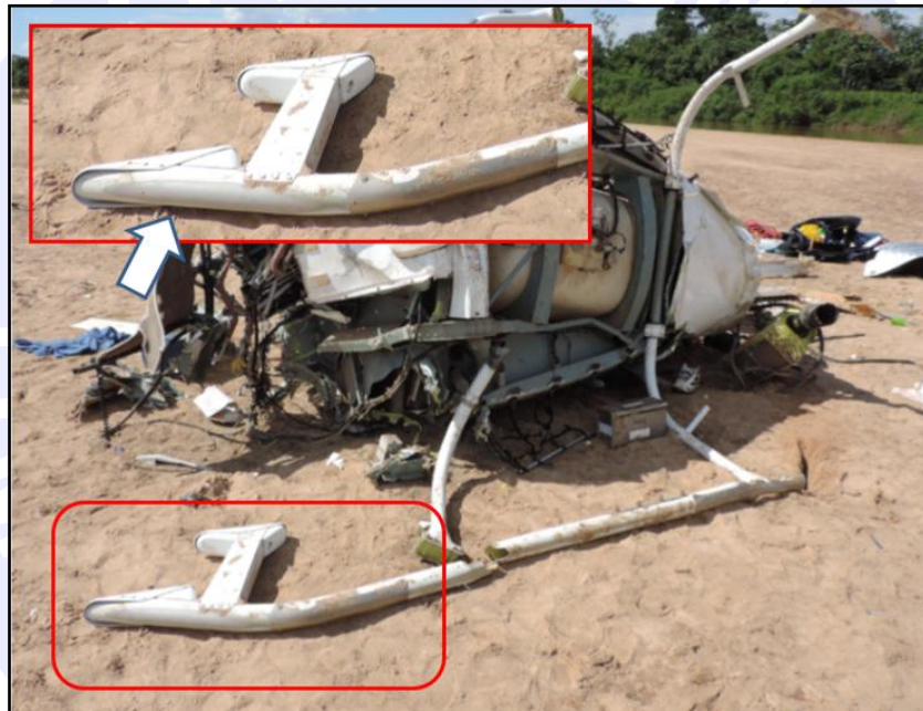
Figure 7 – The end of the right ski, in highlight, was repositioned for evaluation.
