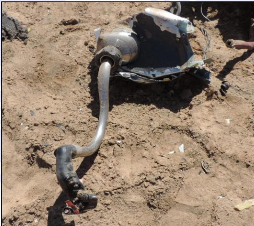
Figure 22 – Cyclic of the right-hand side piloting position, found at a distance of five meters from the aircraft cabin.
