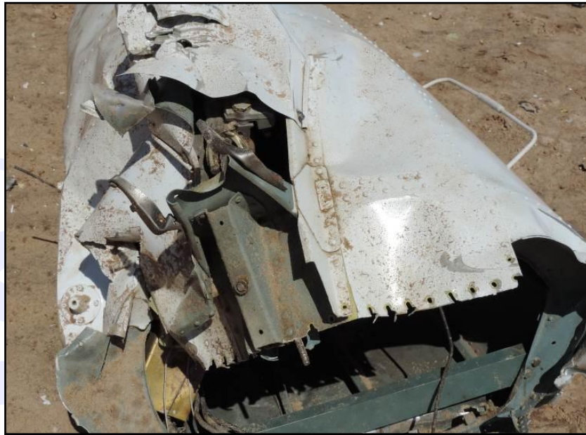
Figure 39 – Section where the breakage of the tail rotor occurred. It is possible to observe that the points of attachment of the rivets were “torn”.
