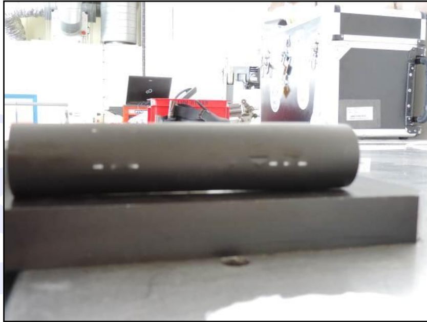
Figure 44 – The central part of the cylinder would not touch the floor surface.
