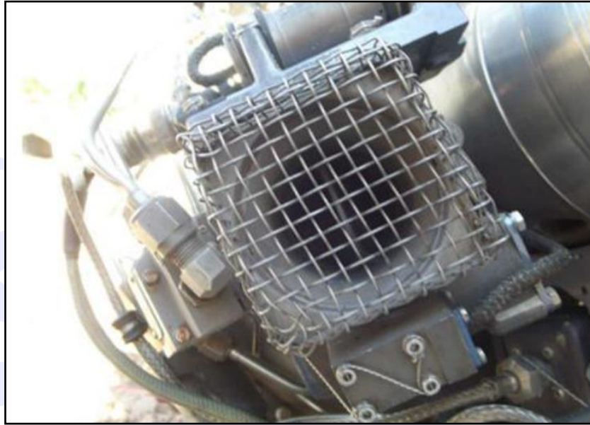
Figure 34 – Bleed valve in the open position.
