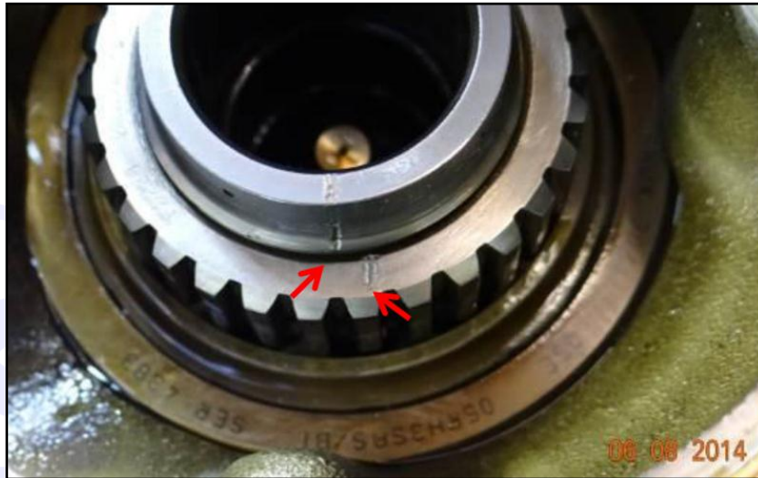
Figure 41 – Misalignment of 2mm in the splined nut of the driving gear.
