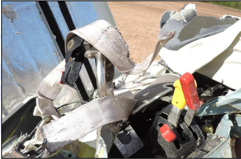
Figure 28 – Abdominal belt of the right front seat with its stitch sewing ruptured.
