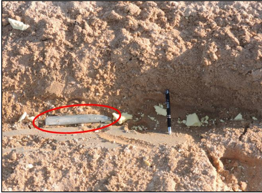
Figure 8 – Point 2: in highlight, the metal component of the tip of one of the main rotor blades.
