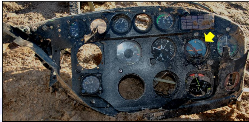
Figure 57 – The aircraft panel detached after the impacts. The artificial horizon is the instrument indicated by the yellow arrow.
