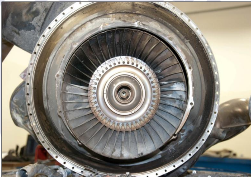
Figure 55 – Front view of the power turbine rotor.
