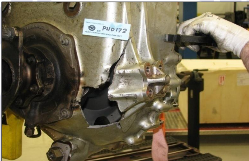
Figure 73 - Fracture resulting from the impact sustained by the RGB in the accident.
