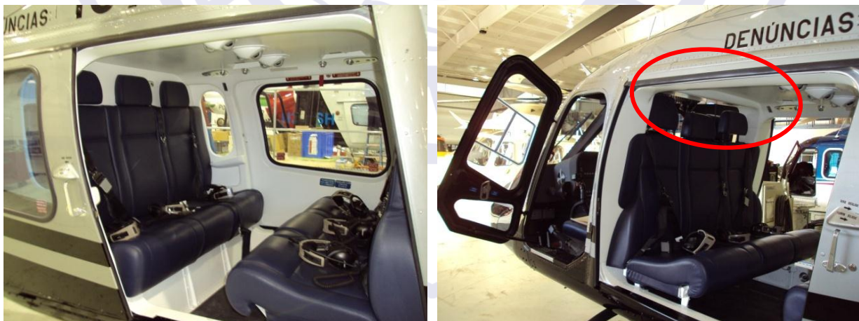
Figures 1 and 2 – Internal configuration of the PP-CGO. The opening between the passengers' cabin and the cockpit is highlighted.
