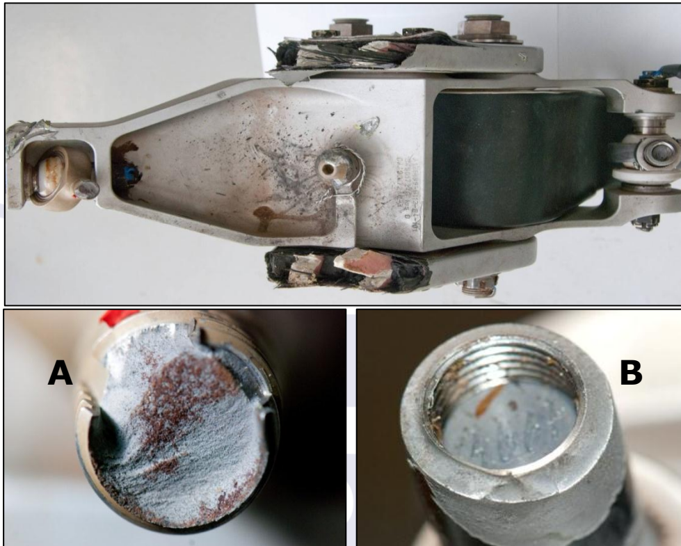
Figures 17, 18 and 19 – Main Rotor propeller blade (blue). The fractures in A and B are characteristic of overload.
