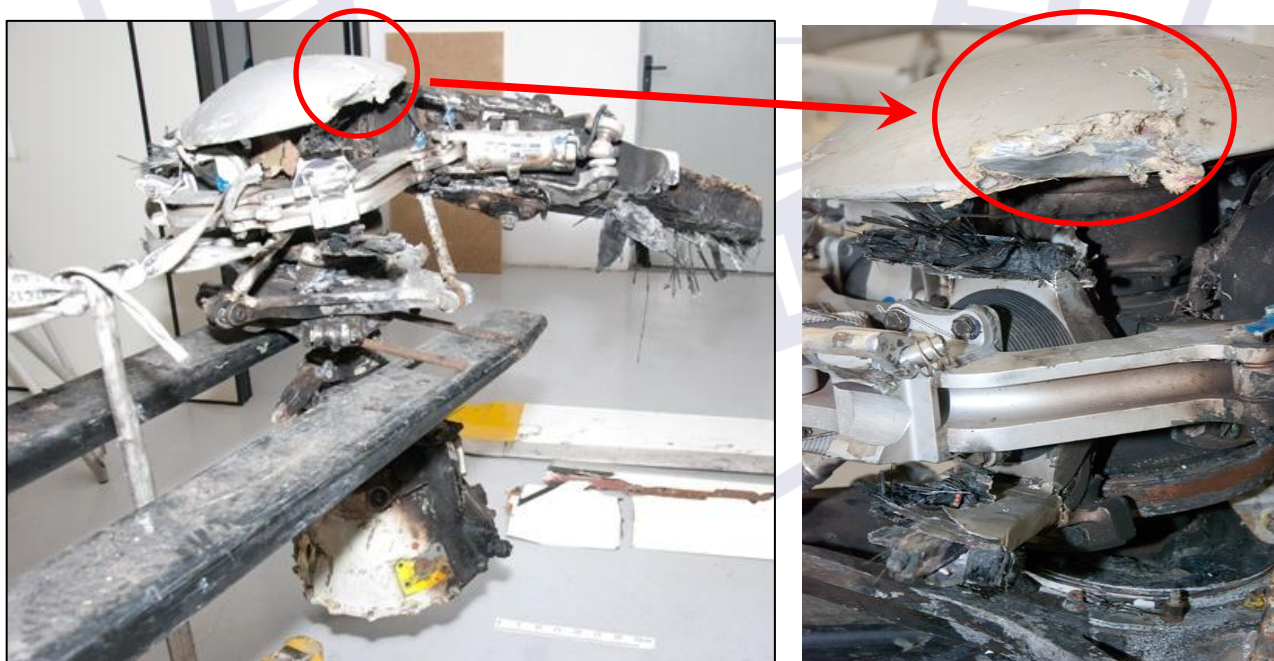
Figures 33 and 34 – Main transmission on the left. On the right, detail of the "Chinese Hat", with a notch probably made by the blue-marking blade's upward vertical movement.
