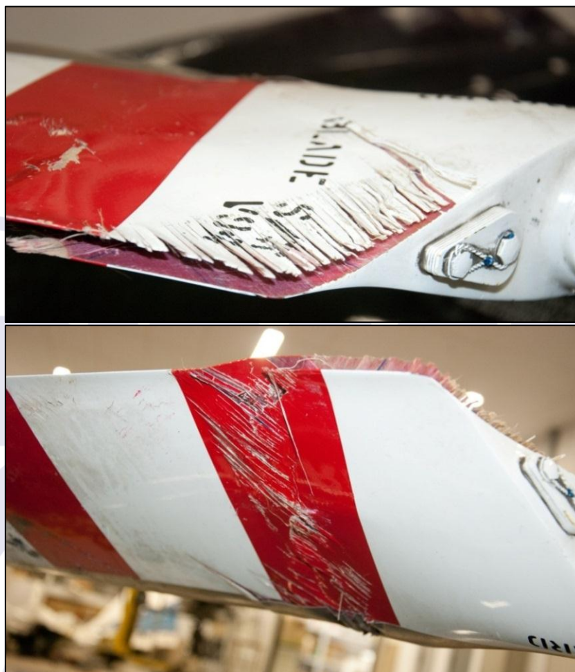
Figures 31 and 32 – Details of the tail rotor blade. The fractures and delamination resulted from the impact with the ground.
