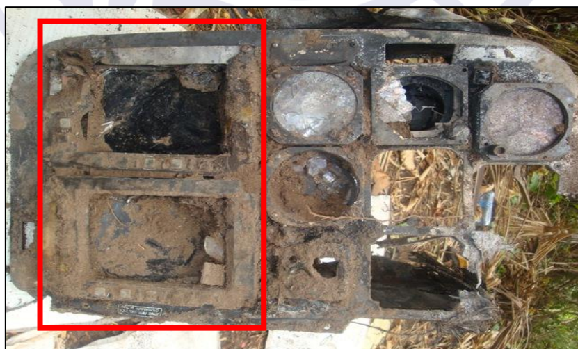
Figure 61 – Panel removed from the wreckage of the PP-CGO. In highlight, the two EDUs taken for analysis in the USA.
