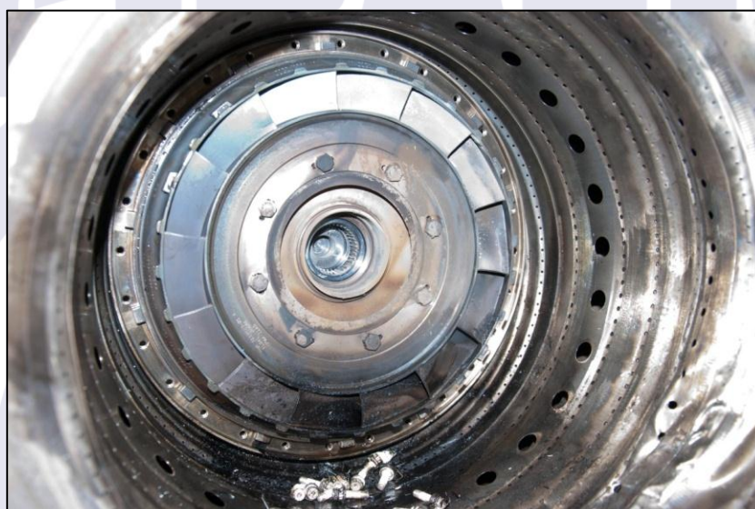
Figure 48 – Compressor Turbine Stator
