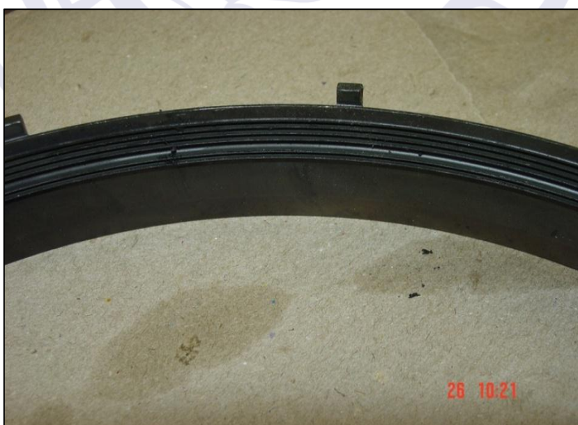
Figure 58 – Detail of the small canals at another point of the sealing ring.
