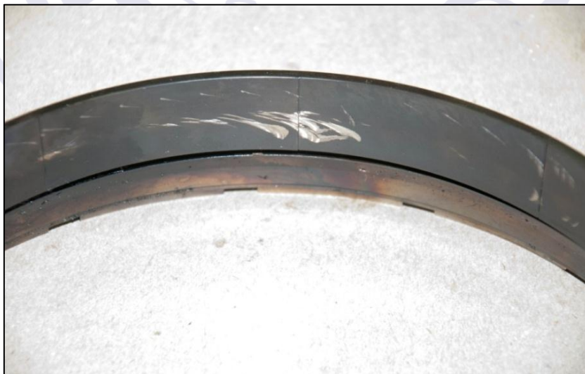
Figure 51 – Marks of impact left by the compressor turbine rotor blades.
