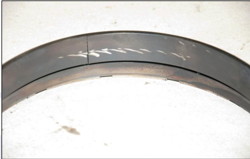
Figure 52 – Marks of impact left by the compressor turbine rotor blades.
