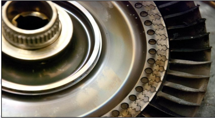
Figure 50 – Marks of mild rubbing at the root of the blades.
