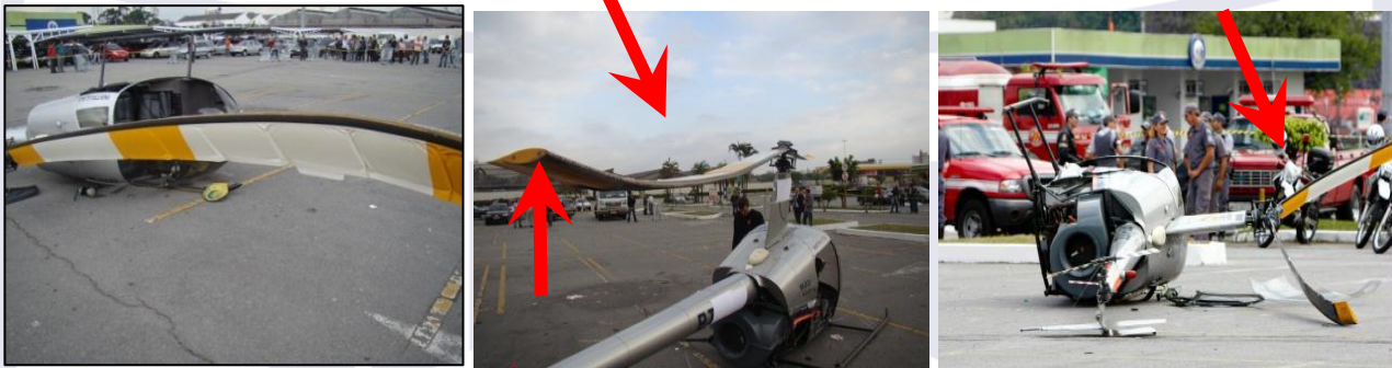
Figures 89, 90 and 91 – Situation of the PT-YZZ main rotor blades after the accident. In highlight, details of the upward bending of the blades. Source: SERIPA IV
