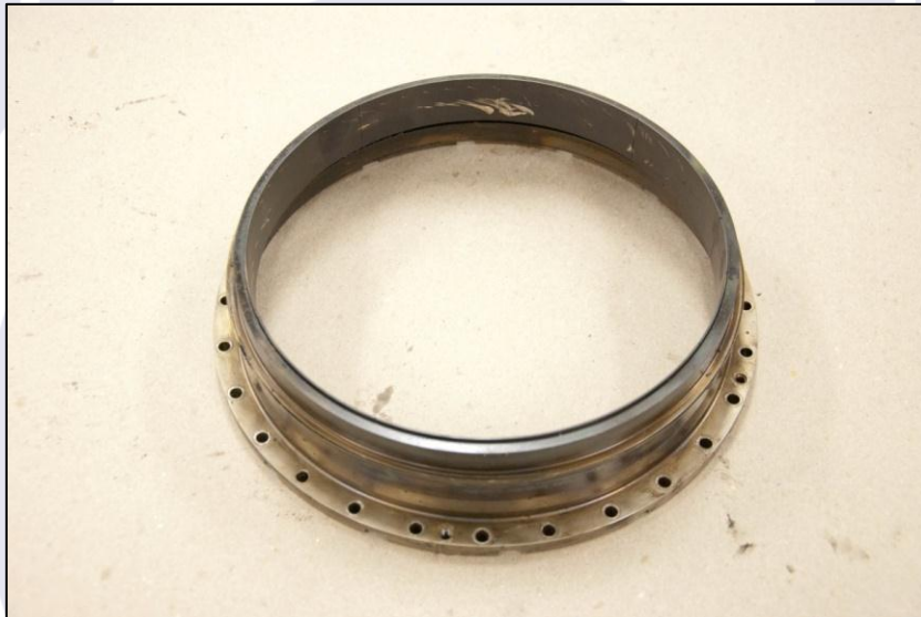
Figure 51 – Segmented ring of the compressor turbine.
