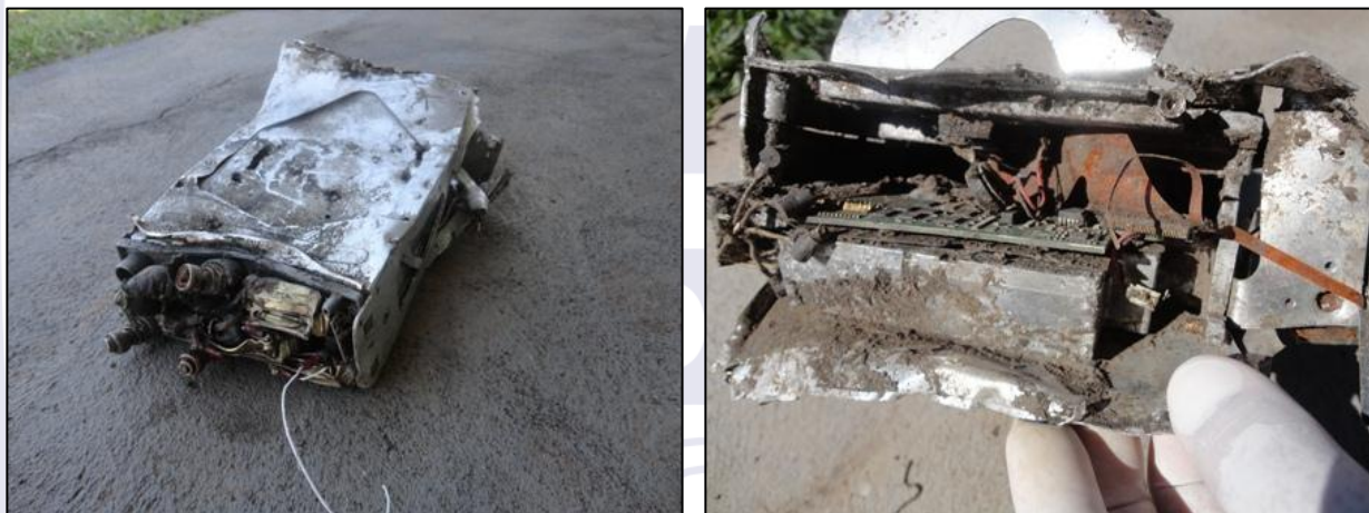
Figures 15 and 16 – Garmin GNS430W GPS equipment retrieved from the PP-CGO wreckage.
