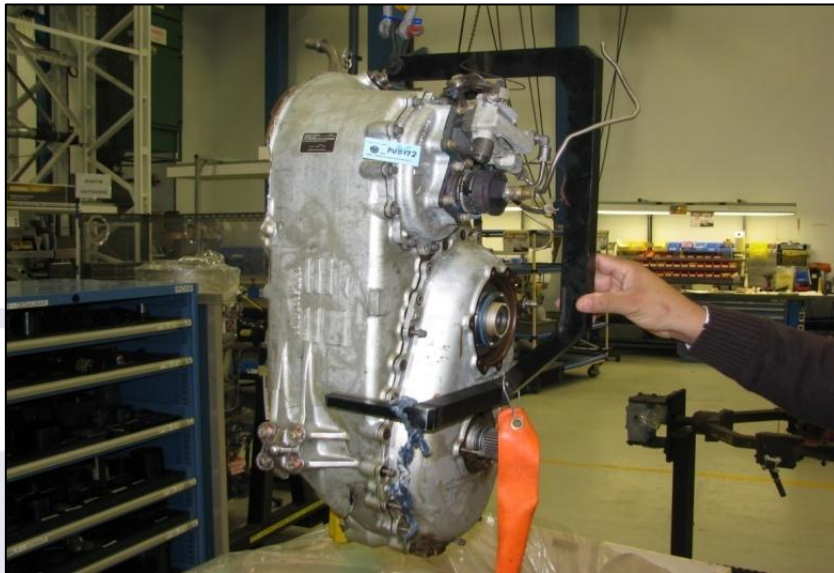
Figure 72 – View of the reduction gear box in the laboratory of analysis of PW Canada.
