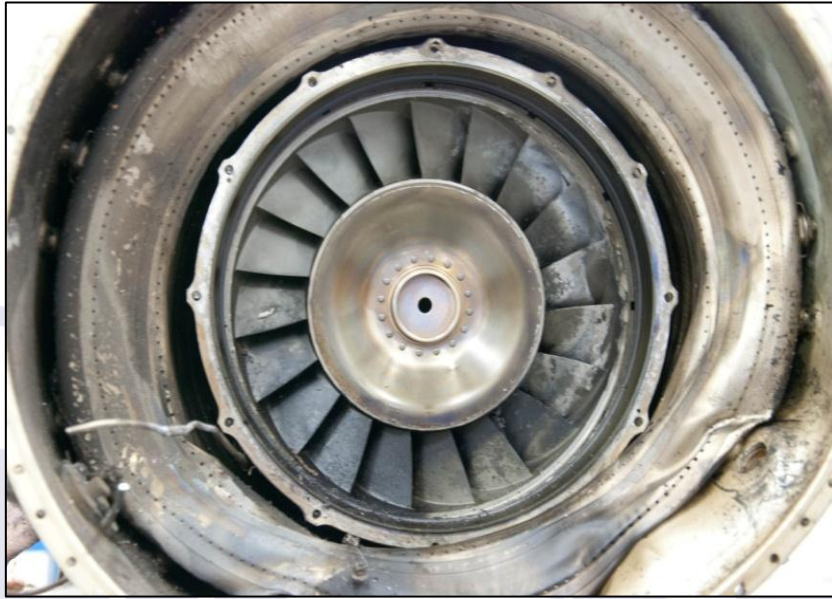
Figure 54 – Back view of the stator of the power turbine with the diaphragm.
