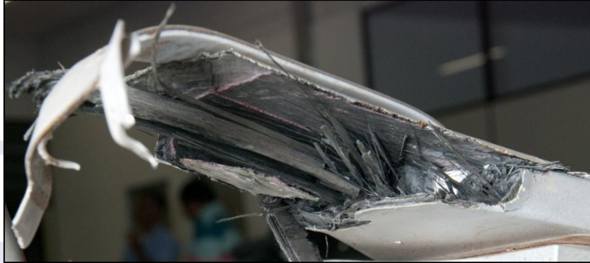
Figures 25 - Fracture details of the red-marking propeller blade.
