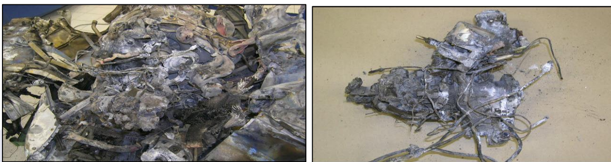
Figures 46 and 47 – On the left, the engine box of accessories. On the right, the High Pressure Fuel Pump and the FCU (Fuel Control Unit) .
