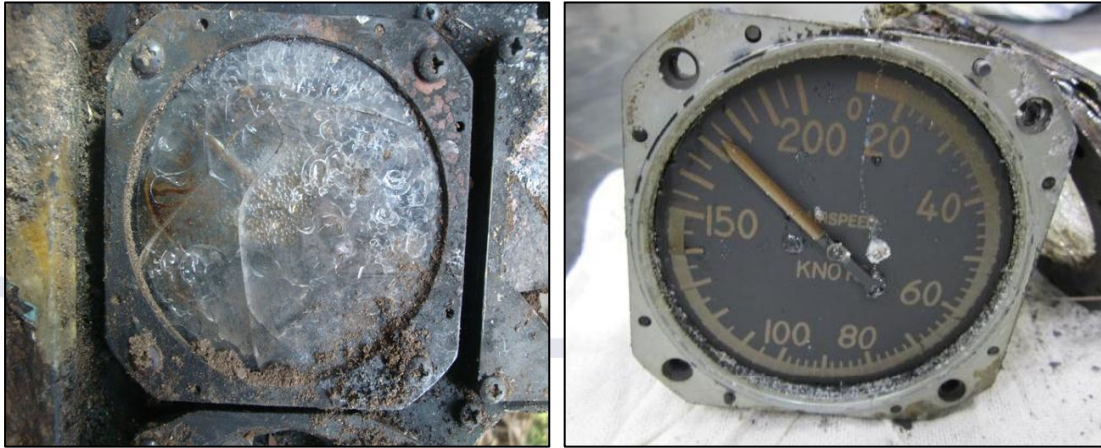
Figures 10 and 11 – ASI of the PP-CGO indicating 174kt. The figure on the right shows the same instrument, after removal of the glass broken in the impact.
