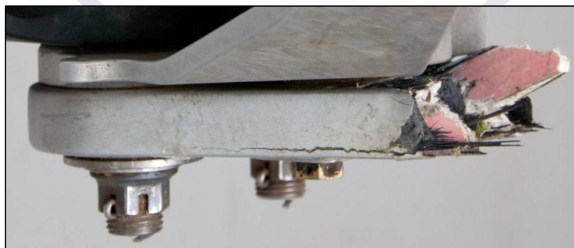
Figure 24 - Detail of the fracture as viewed from the bottom. It is possible to see regions of compression and traction on the surface of the fracture.
