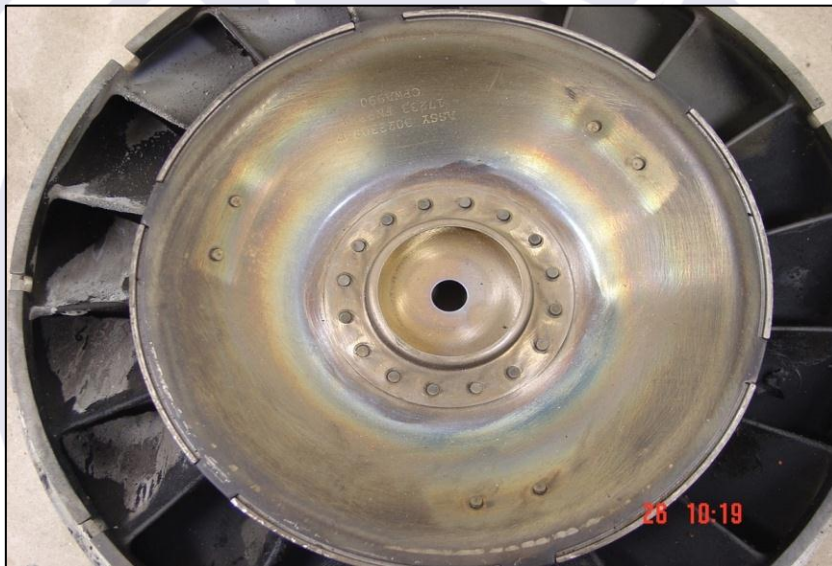
Figure 53 – Diaphragm with marks of light rubbing left by the roots of the compressor turbine rotor blades.
