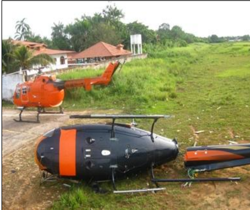
Figure 1 - Approaching view of PR-RCH (behind, there is the other aircraft hit in the tail rotor).
