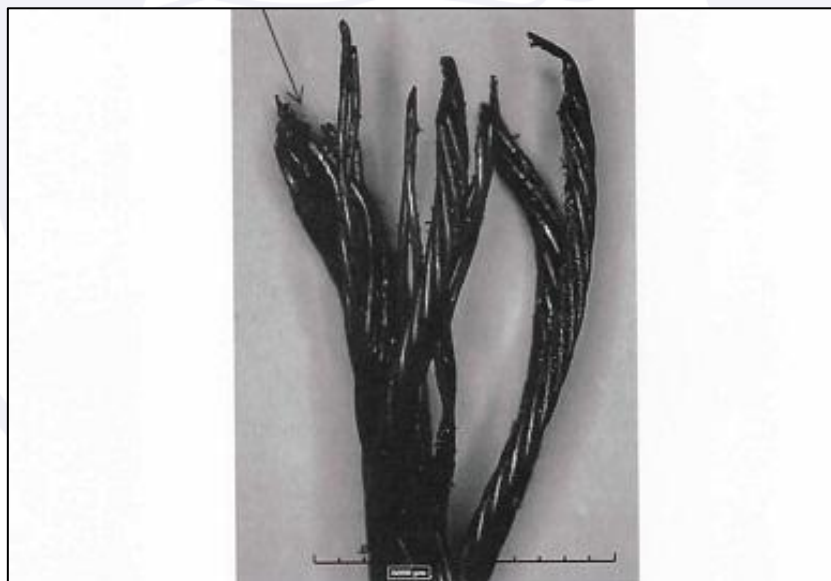
Figure 3 – Aspect of the elevator trim cable rupture due to overload.
