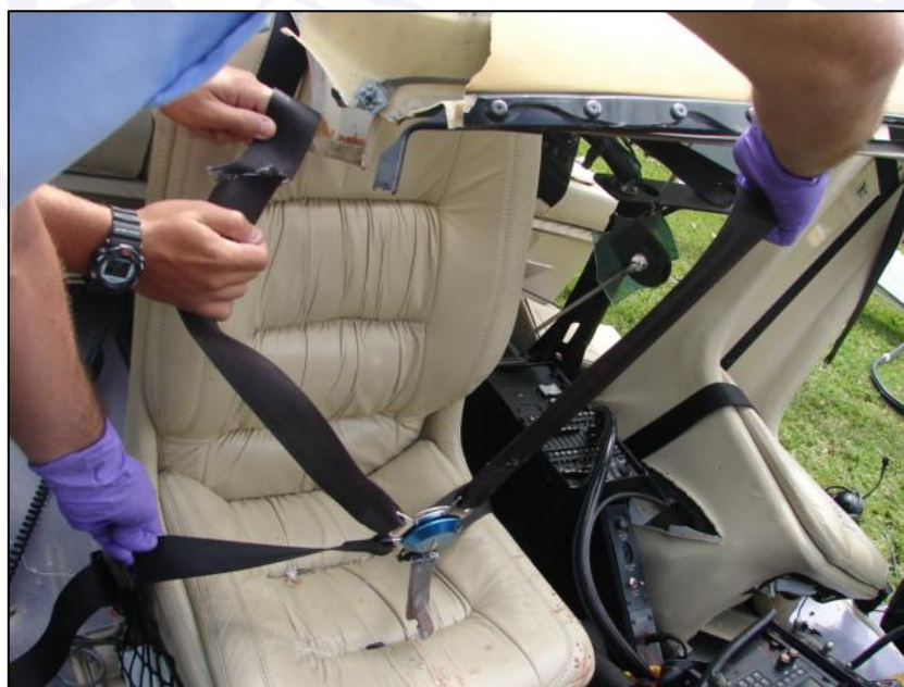
Figure 2 – Aspect of the pilot's seat belt after the impact.
