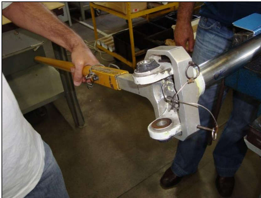
Figure 21 – Application of torque on the bolt by means of a torquemeter.
