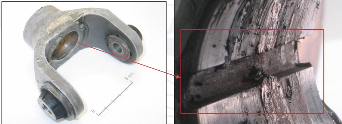
Figure 6 – Support fork of the PT-YRE blades (left). On the right, the inner surface of the fork, showing the groove for the 'tongue' in highlight.
