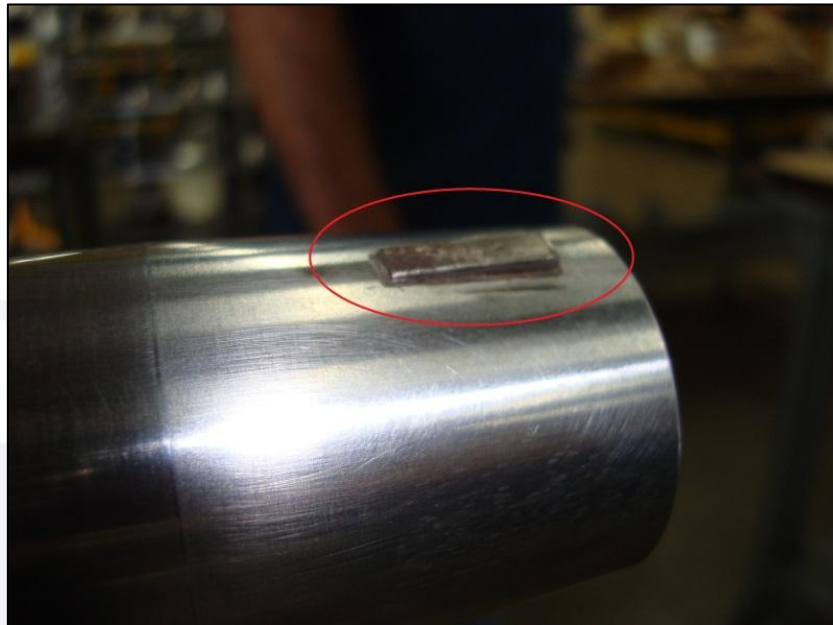
Figure 5 – Transmission shaft ready to be installed. In the highlight, the tongue on the surface of the shaft.
