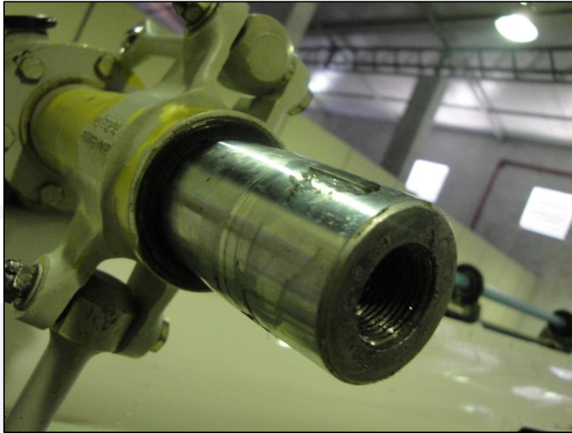
Figure 29 – ‘Tongue’ showing loss of material, after application of torque simulating turn.
