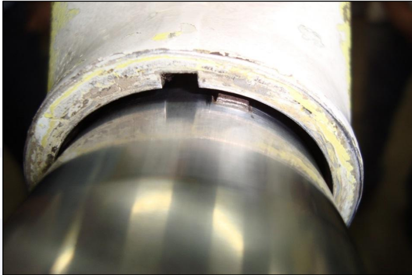
Figure 23 – Incorrect installation of the fork in the conical shaft.
