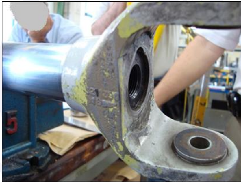
Figure 17 – Fork installed in the conical shaft.
