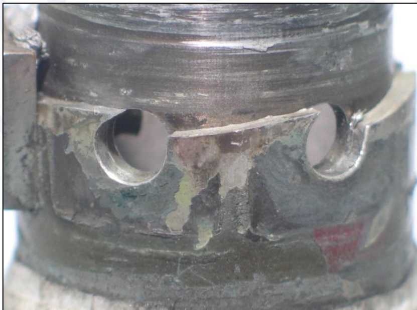
Figure 14 – Failure observed in the long shaft. The slope of the fracture indicates that there was overload due to torsion.
