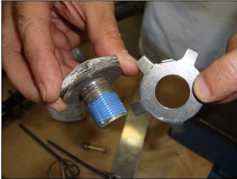
Figure 22 – Application of Loctite on the bolt, before setting the final torque.
