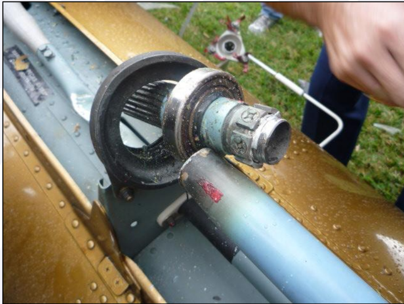
Figure 13 – Rear transmission, as found at the Initial Action.
