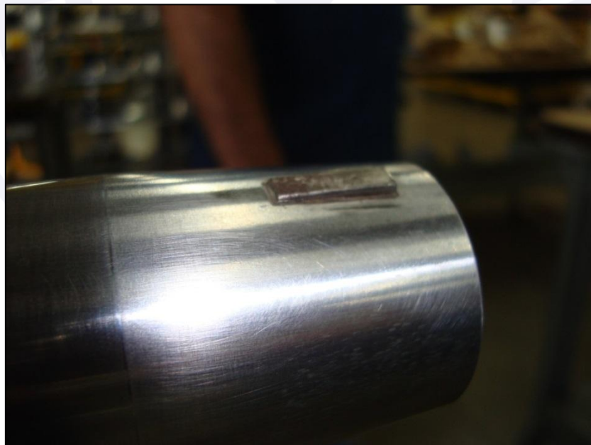
Figure 28 – 'Tongue' installed before the application of torque simulating turn.
