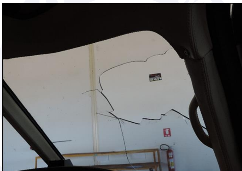
Figure 1 - Internal view of the right windshield damaged by the impact against the vulture.
