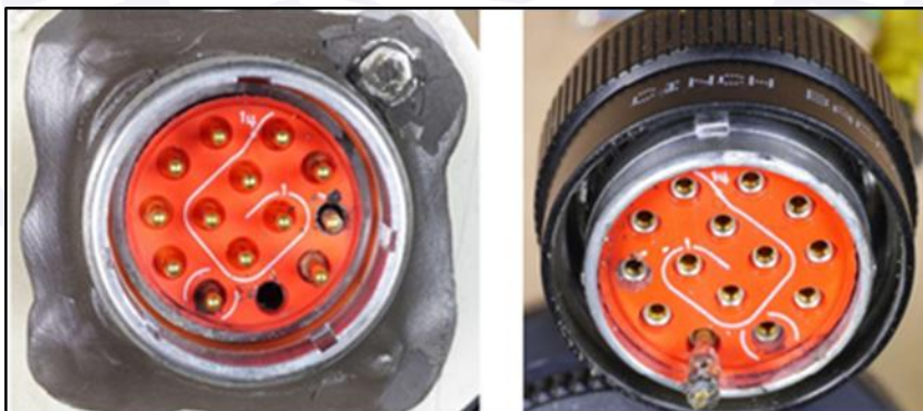
Figure 26 - On the left the D7232P connector and on the right the D7232J connector.
