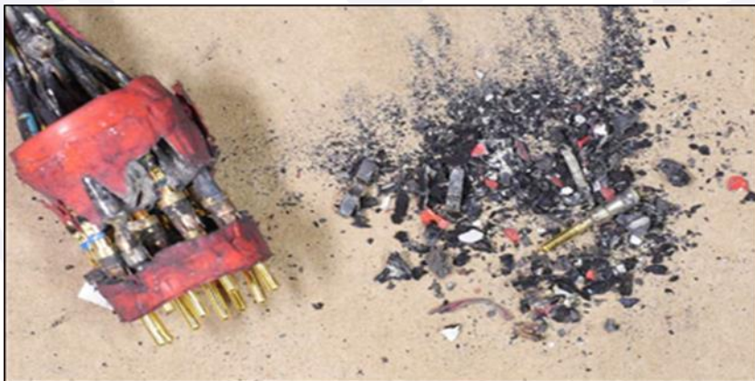
Figure 29 - Fragmented material from the disassembly of the D7232P connector.
