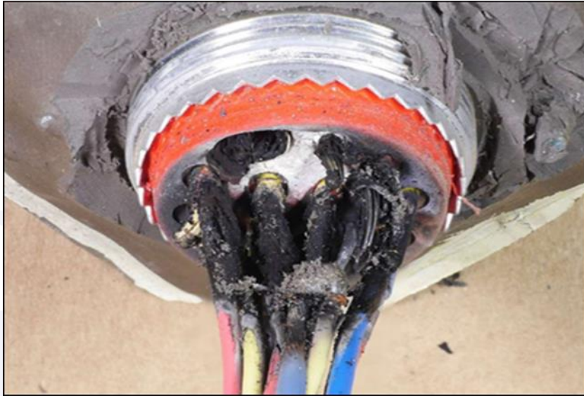
Figure 27 - D7232P connector after removing the housing.
