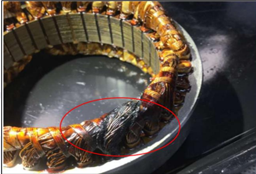
Figure 13 - Damage to the PMG stator.
