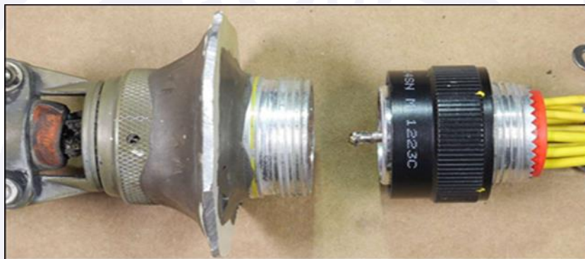
Figure 25 - Separation of the connector D7232P/J.
