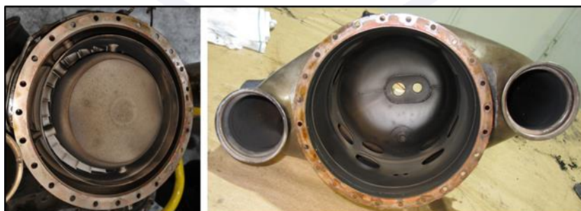
Figure 60 - Shield, stators and combustion chamber case.
