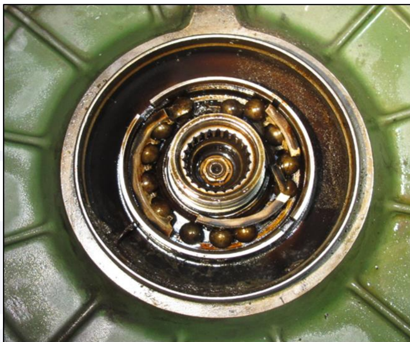
Figure 44 - Bearing nº 2 with the fractured ball separator.
