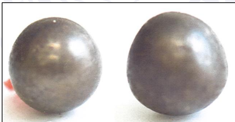
Figure 46 - Balls of bearing nº 2 worn and ovalized.
