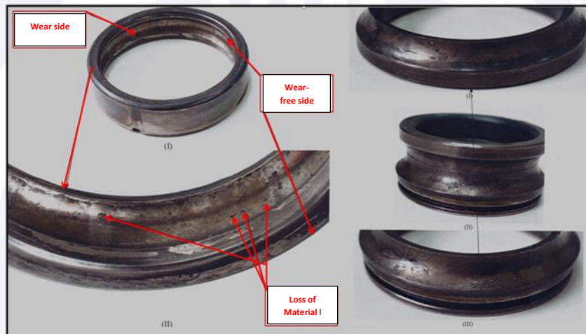
Figure 48 - External and internal tracks with wear and loss of material.
