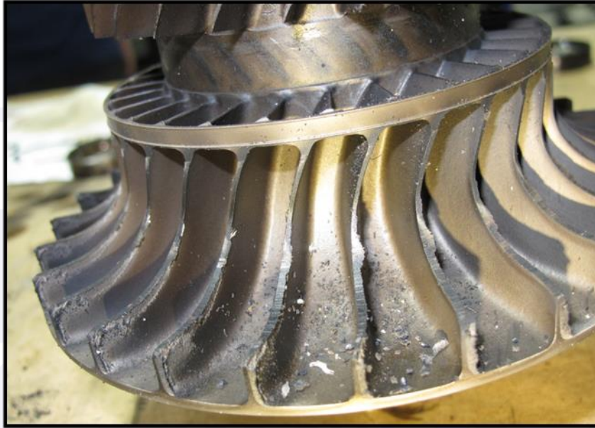
Figure 42 - Loss of material from the centrifugal compressor impeller.
