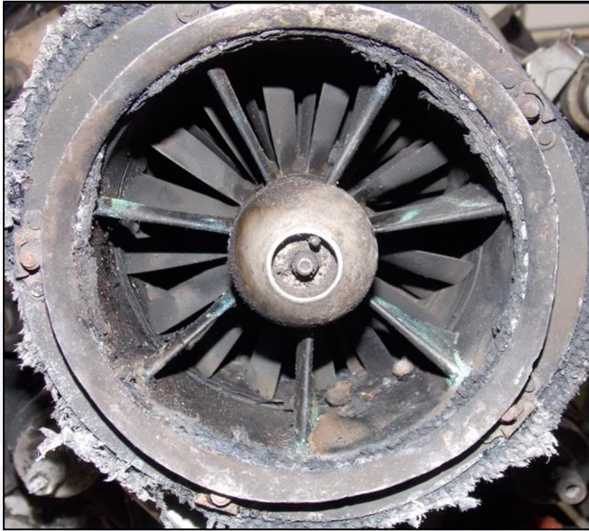
Figure 39 - Front view of the axial compressor air intake.
