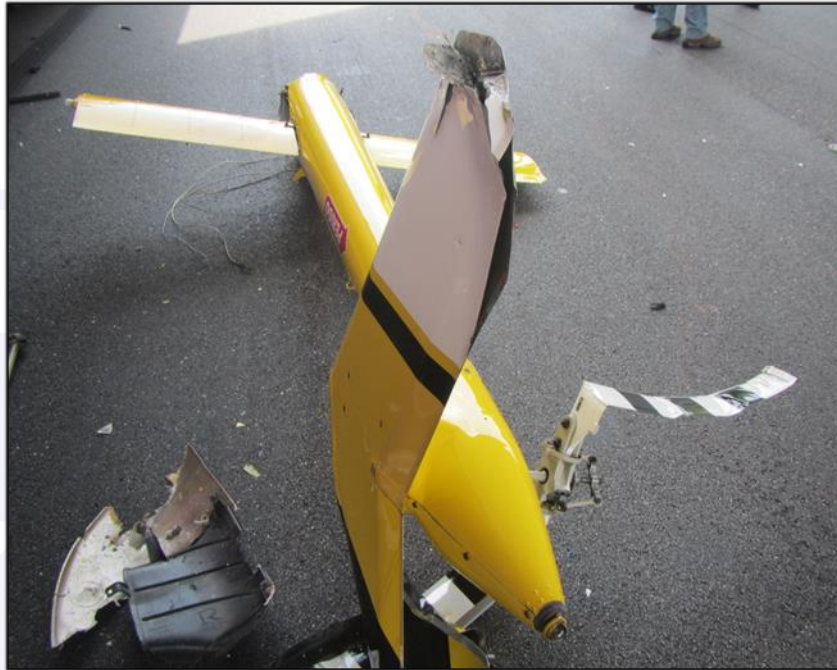
Figure 2 - Sectioned tail boom.
