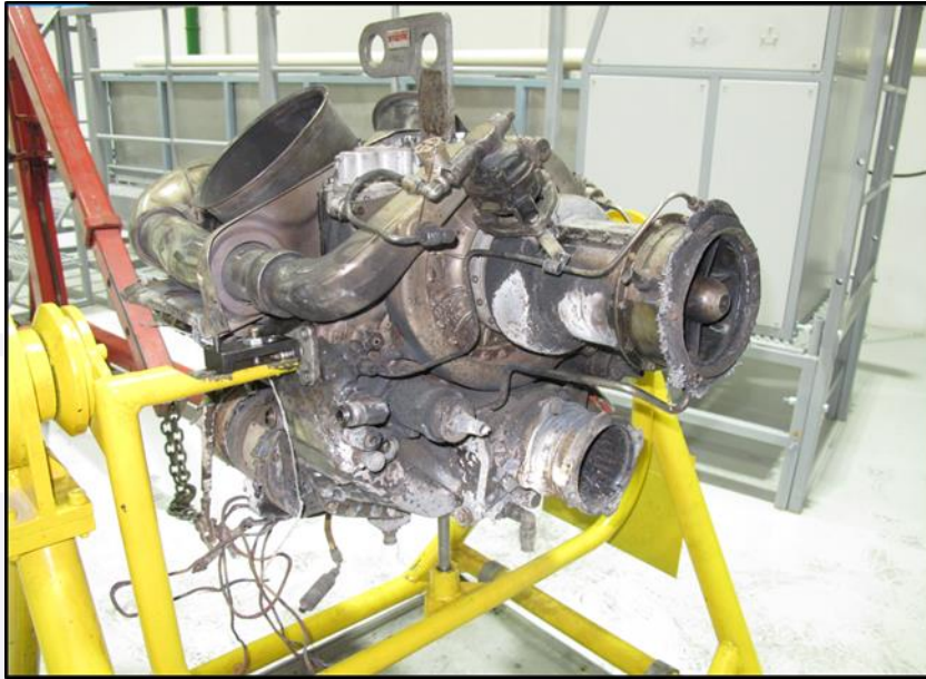
Figure 37 - External condition observed in the engine that equipped the PT-HPG aircraft.
