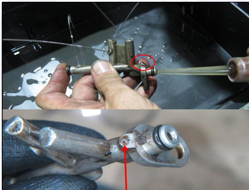
Figure 53 - The oil delivery tube with blocked orifice.
