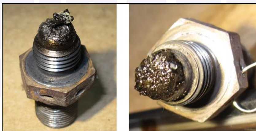
Figure 50 - Metallic material deposited on the Magnetic Chip Detectors.
