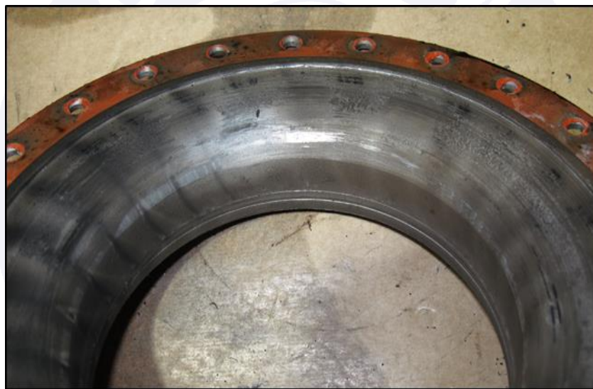
Figure 43 - Scratch marks on the centrifugal compressor housing (Shroud).
