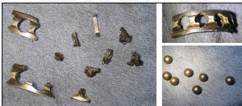
Figure 45 - Fractured ball separator.
