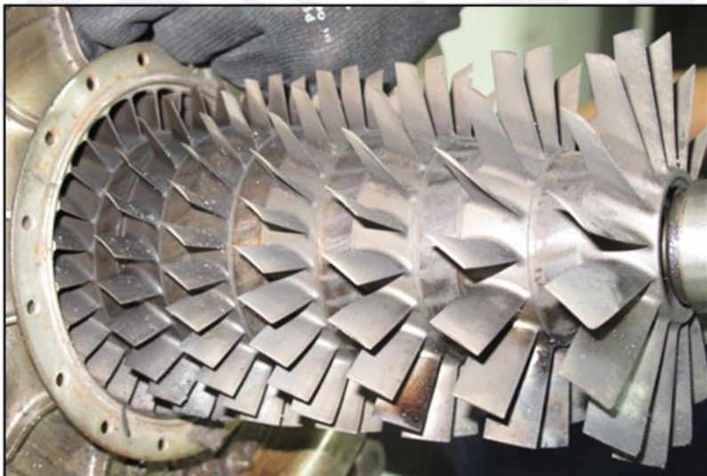
Figure 41 - Rotor blades intact (axial compressor impeller).
