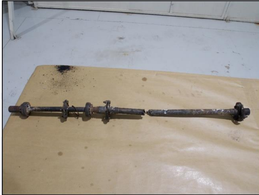
Figure 34 - Connecting shaft between the “Gearbox” and the tail rotor.
