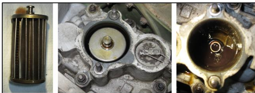
Figure 49 - Oil pressure filter and the filter container.
