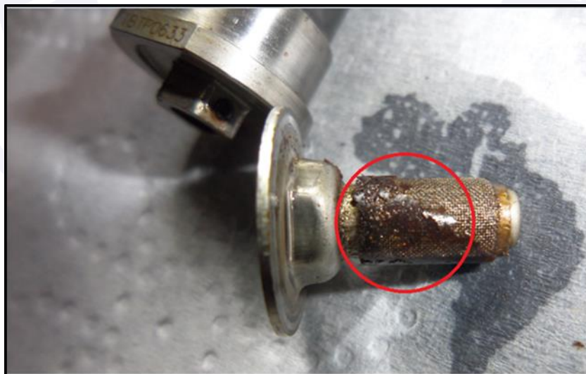
Figure 4 - Contaminated Fuel nozzle highlighted.
