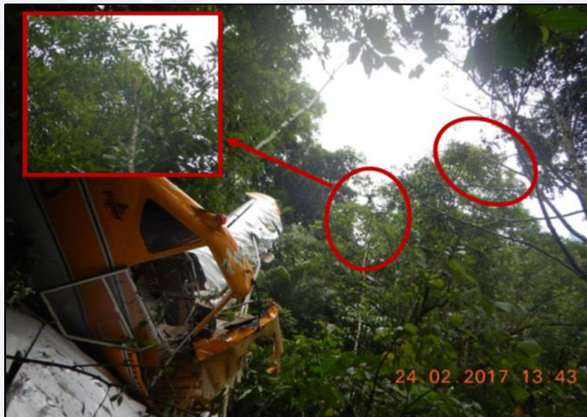
Figure 2 - View of the location of the aircraft collision and impacts on the vegetation.
