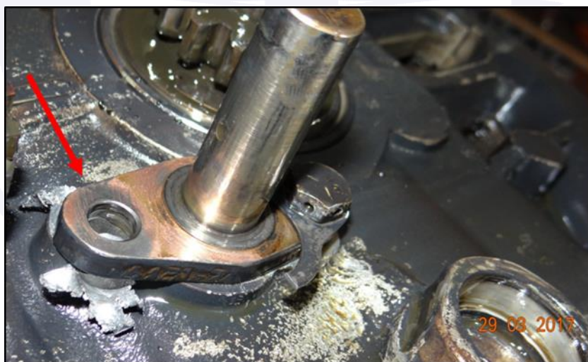
Figure 6 - Detail of the absence of the fixation stud of the left magneto drive gear and the valve control.
