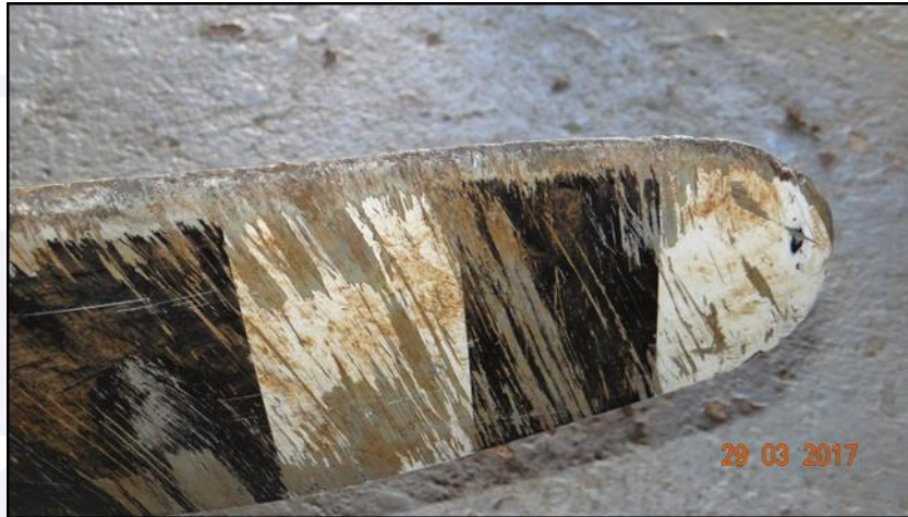
Figure 5 - Impact marks on the leading edge and transversal hazards on the back of the blade.
