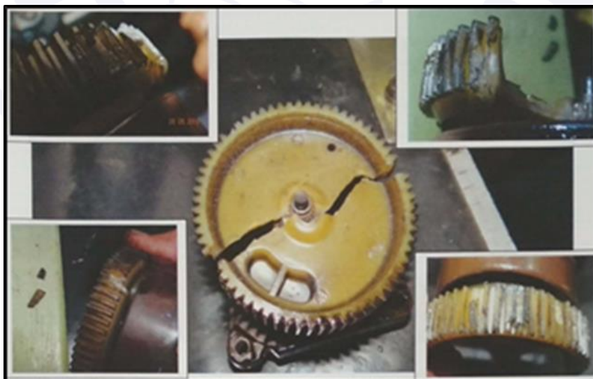
Figure 6 - View of the gear and the various distal teeth of the left magneto damaged by dents or fractures.
