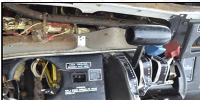
Figure 5 - Approximate view of the center console, with the levers and its positions.
