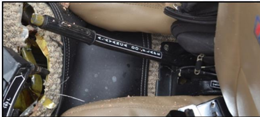
Figure 4 - View of the interior of the aircraft. It has been checked the position of the control lever of the flaps in the totally retracted position.
