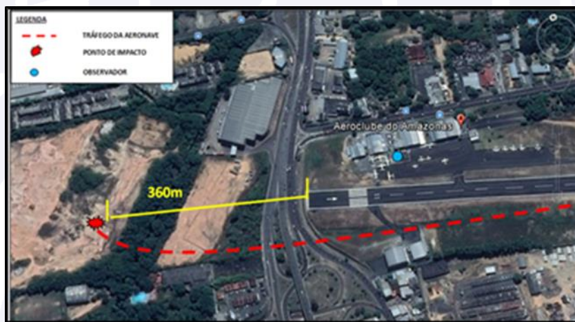
Figure 1 - Sketch of the accident, showing the air view of the impact site and its position in relation to the SWFN threshold 11. The dashed red line shows the route covered by the aircraft until the moment of impact.
