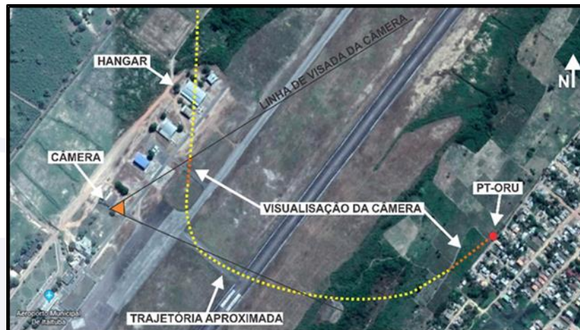
Figure 2 - Sketch of the accident, with the line of sight of the safety camera and approximate trajectory of the aircraft until the impact.
