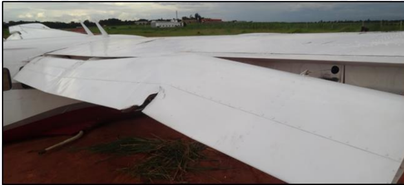
Figure 3 - Damage to the flaps.
