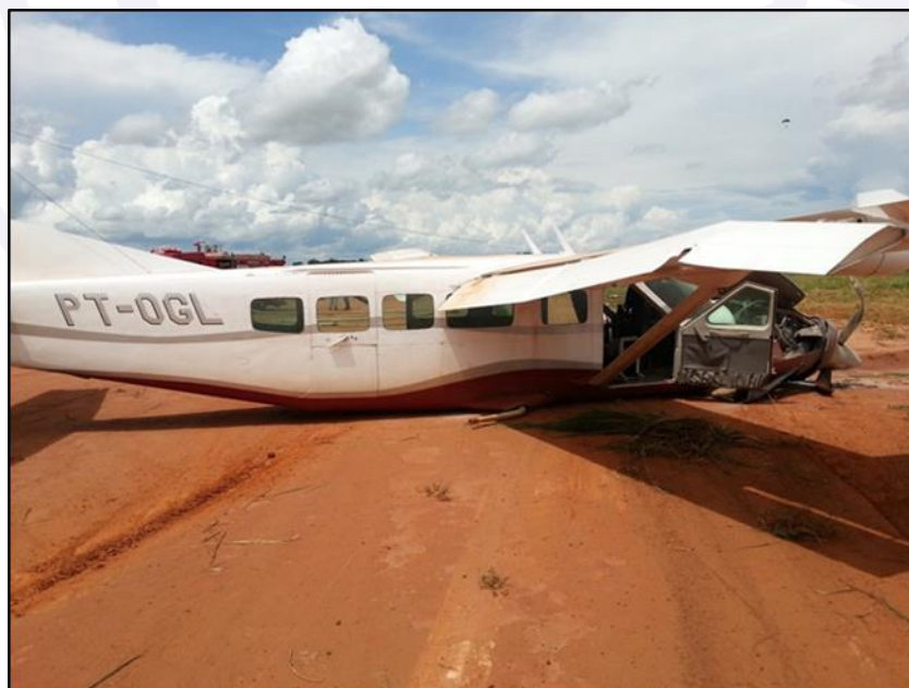
Figure 1 - Overview of the aircraft, with damage to the propeller, flaps and landing gear.
