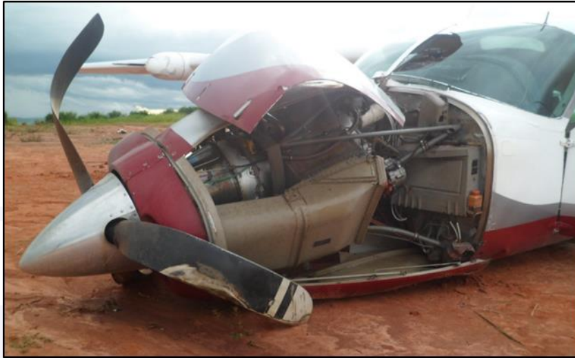
Figure 2 - Damage to the propeller, engine and left windshield.
