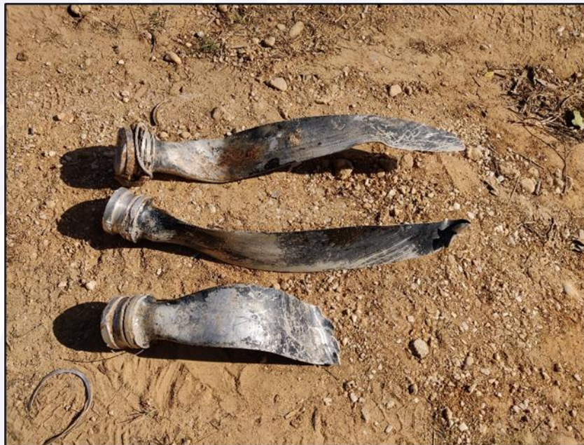
Figure 2 - Propeller blades with torsions and ruptures typical of power impact.
