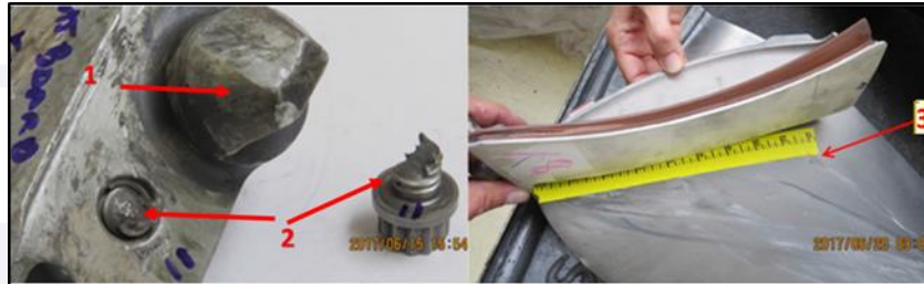
Figure 13 - Annulus filler: post (1) and screw (2). Brands on Blade (3).
