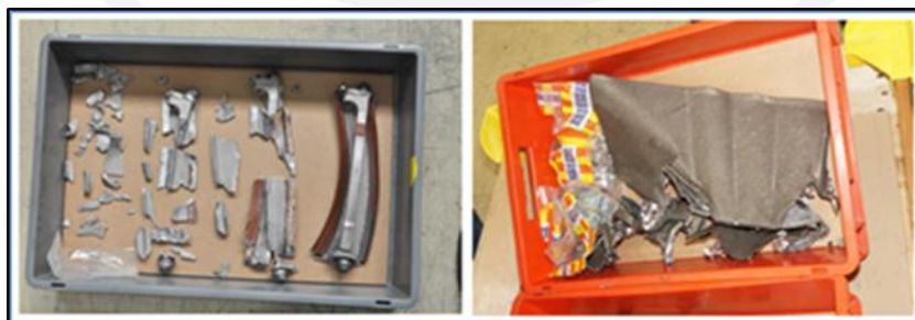
Figure 12 - Parts and fragments of the engine sent separately for analysis.
