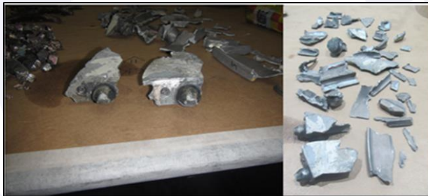
Figure 8 - Annulus filler that separated from the engine.
