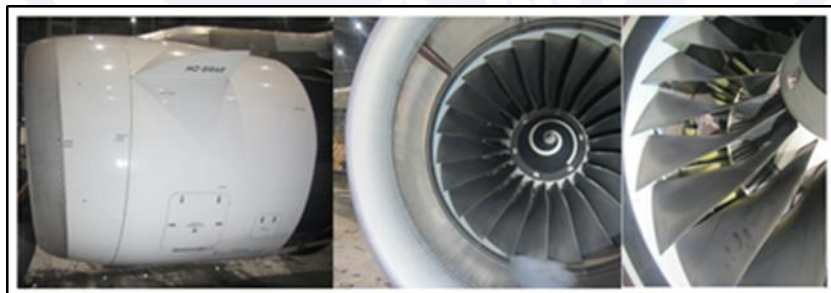
Figure 2 - Right engine overview, air intake and detail of external damage.
