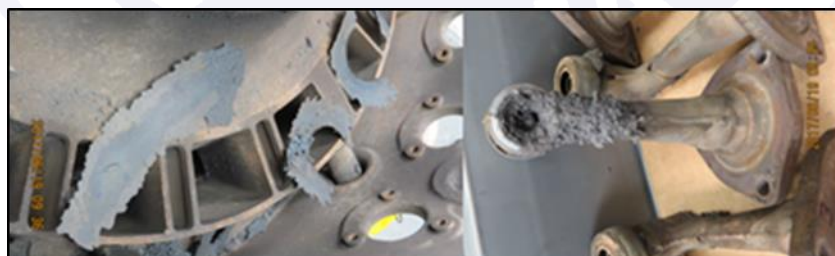
Figure 15 - Diffuser housing and fuel nozzle with melted debris.
