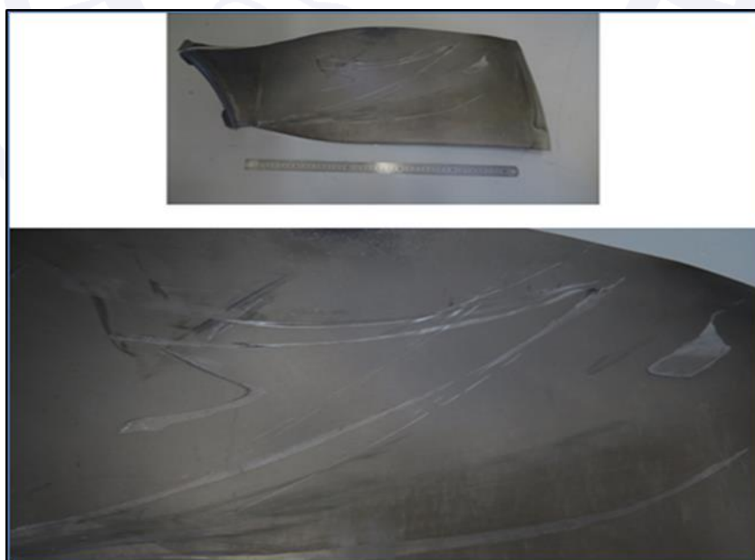
Figure 5 - Detail of damage to one of the blades.
