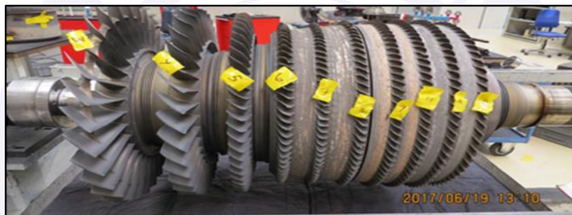
Figure 14 - Fractured blades of the high-pressure compressor.
