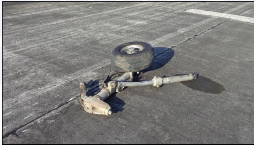
Figure 10 - Left landing gear with the actuator cylinder.
