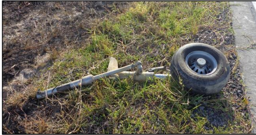
Figure 9 - Right main landing gear with the actuator cylinder.
