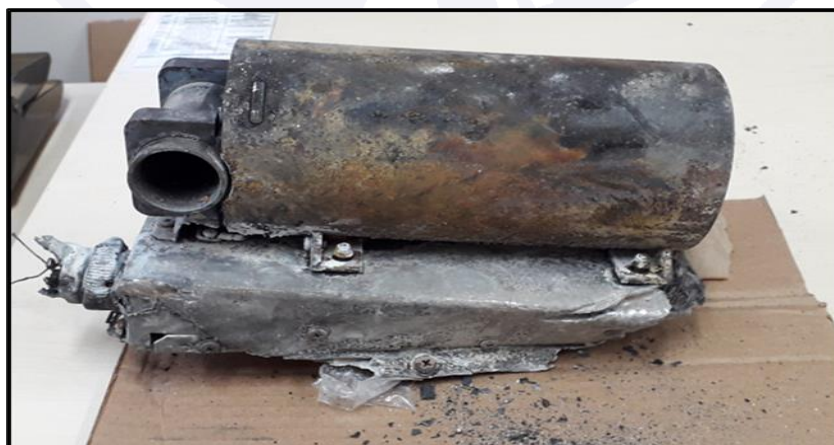
Figure 6 - Cockpit Voice Recorder that equipped the aircraft.
