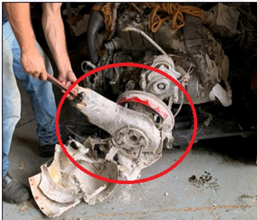
Figure 9 - Detail of the root of the blade that remained attached to the shaft.
