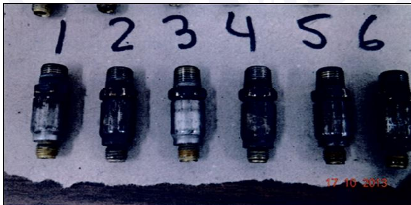
Figure 6 - Overview of the right engine nozzles.
