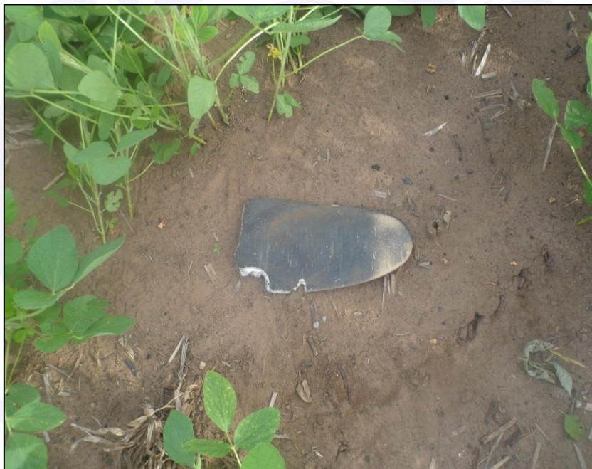
Figure 4 – Fragment of the propeller blade found near the concrete pole hit by the aircraft.
