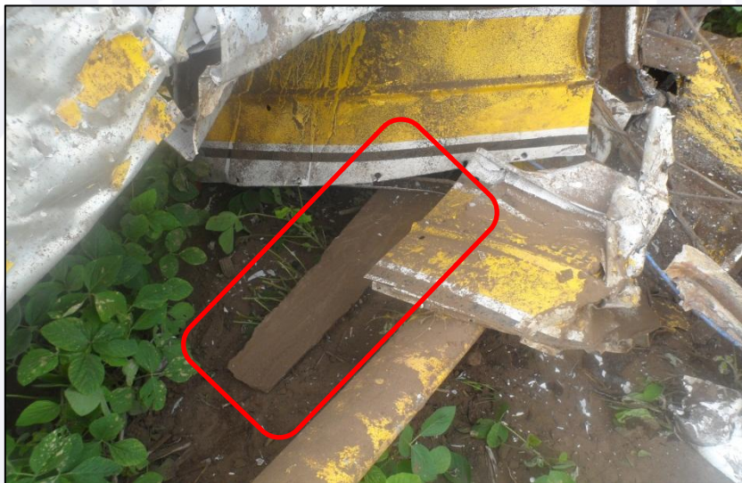
Figure 2 – Fragment of the concrete pole amid the aircraft wreckage.
