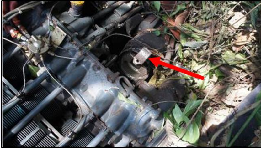
Figure 3 - Block of the engine fractured at the base of cylinder # 2 and head of the fractured connecting rod.
