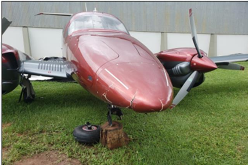
Figure 2 - Damage to the nose section and auxiliary landing gear.
