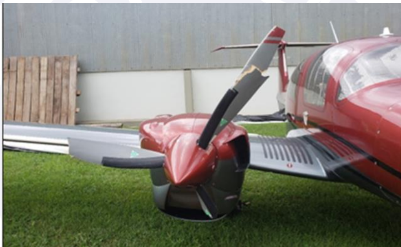
Figure 3 - Damage to the right engine propeller assembly.
