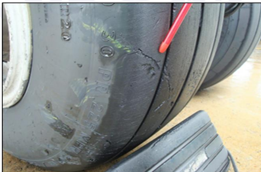
Figure 10 - Damage to the tire of the left main landing gear.
