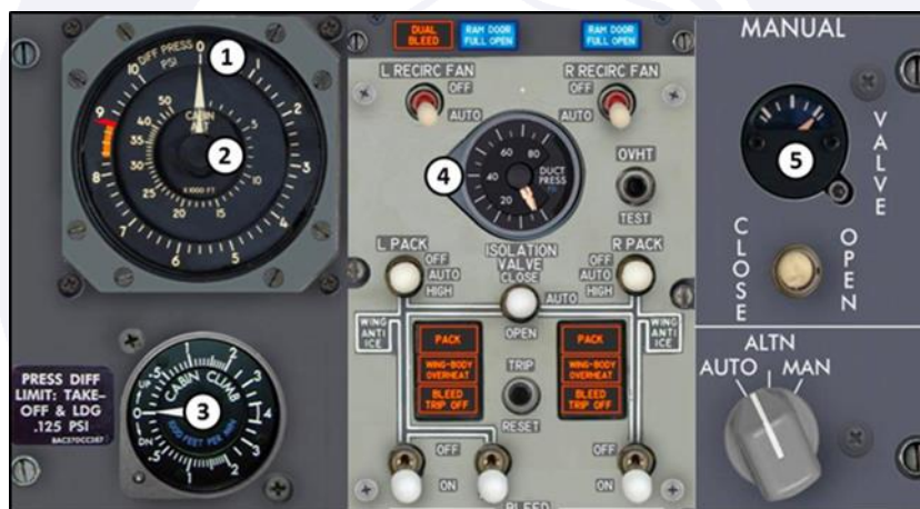
Figure 3 - Overhead Panel cutting with the pressurization and air conditioning system control panel indicators: 1 - pressure differential; 2 - cabin altitude; 3 - ramp up / down ratio; 4 - pressure in the pneumatic ducts; and 5 - Outflow valve position indicator.
