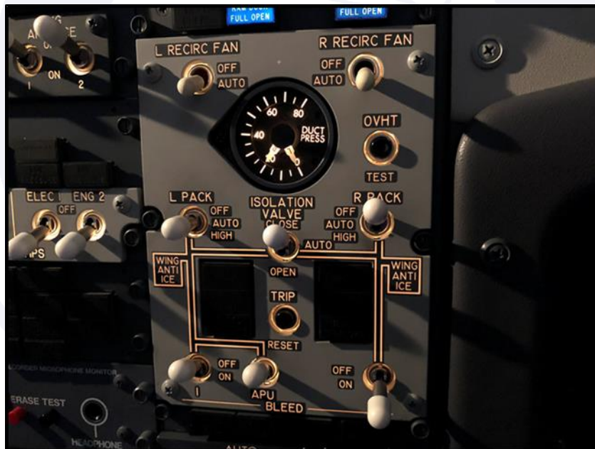
Figure 9 - Pressurization panel of a B737-800 flight simulator, reconstituting the configuration adopted after take-off.
